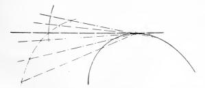
the given point and some on the other. About the given point as center with any convenient radius strike a circular arc, crossing such region as it is judged the tangent will pass through. On each secant at a distance
