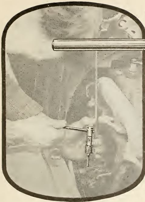
Tapping for new bolt in exhaust pipe bracket
