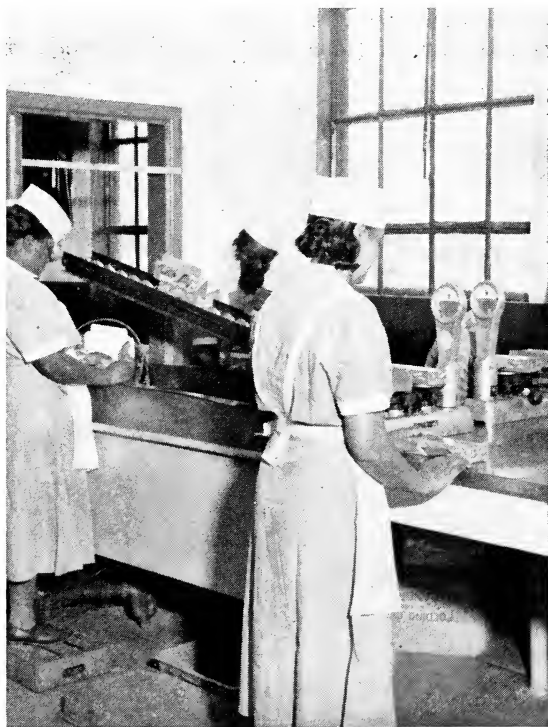
Figure 12.4. Checking weight of packaged raw shrimp prior to freezing. ( "Fish Boat," H. L. Peace Publications. )
