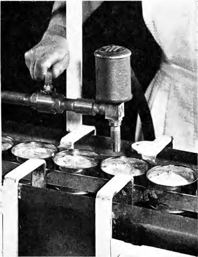
Figure 7.7. Regulating vegetable broth addition to filled cans. Solenoid valve cuts flow when line is stopped. ( Westgate-California Corporation. )
