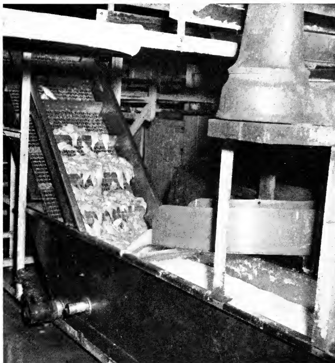
Figure 5.2. Escalator conveyor carrying ocean perch fillets out of brine tank. ( F. T. Piskur, U.S. Fish and Wildlife Service. )
