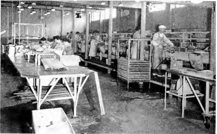
Figure 22.4. Filleting room of a Pacific Coast processing plant. The filleting line is at the right and the packing line at the left. ( Whiz-Eardley Fisheries Co. )
