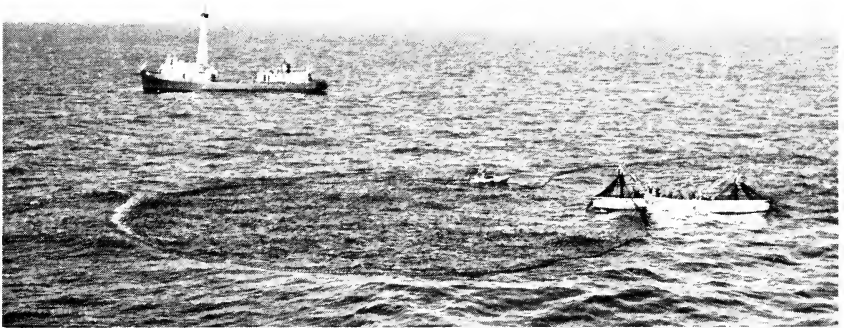
Figure 11.1. Menhaden purse seine in operation. The wings of the seine are being hauled aboard the two purse boats by power-driven blocks. After the fish have been concentrated in the bunt, the carrier vessel will move along side for transfer of the catch into the hold.
