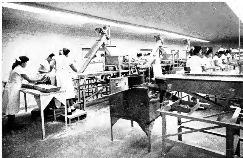
Figure 12.5. Breading of raw shrimp. The breading line is on the left, the packing lines on the right. ("Fish Boat," H. L. Peace Publications.)
