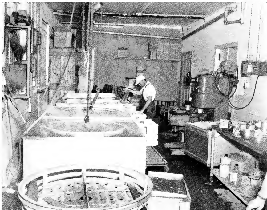
Figure 14.2. Pasteurization of blue crab meat in an East coast plant. Open tanks can be used since the cans of crab meat are pasteurized at a temperature well below the boiling point of water. The tanks in the background are used to cool the cans. ( U.S. Fish and Wildlife Service. )
