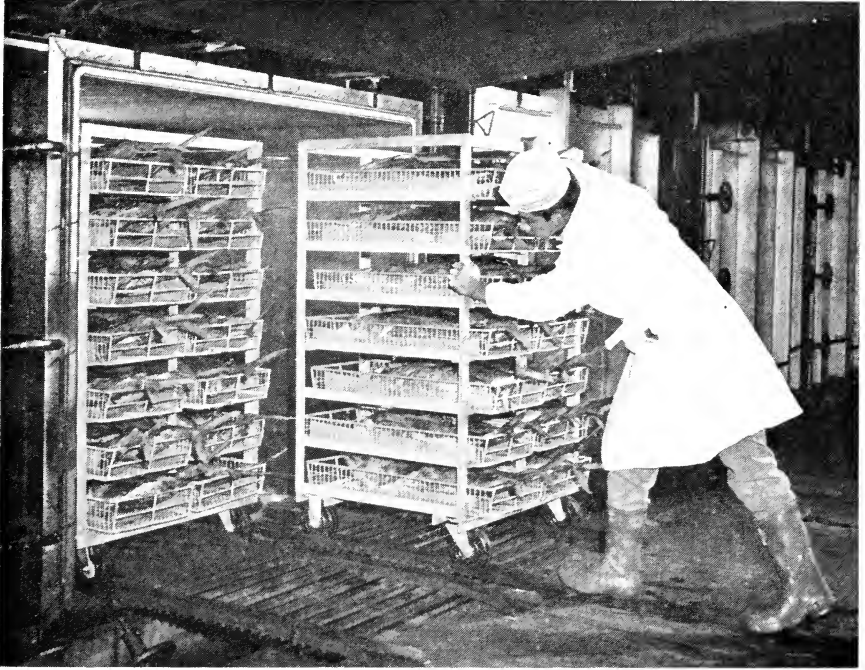
Figure 7.4. A rack of raw tuna being wheeled into the cooker. ( Westgate-California Corporation. )
