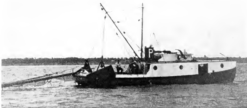
Figure 6.3. Stern-type trawler, typical of several that have been developed from traditional gill net tugs.
