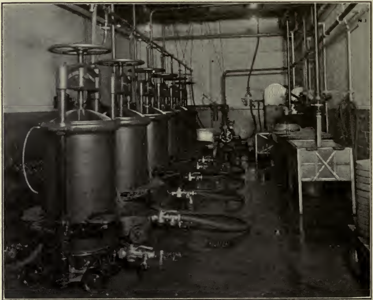
Fig. 47.—Filter Presses for Clarifying Beer before Bottling. (Courtesy of United States Brewers' Association.)
