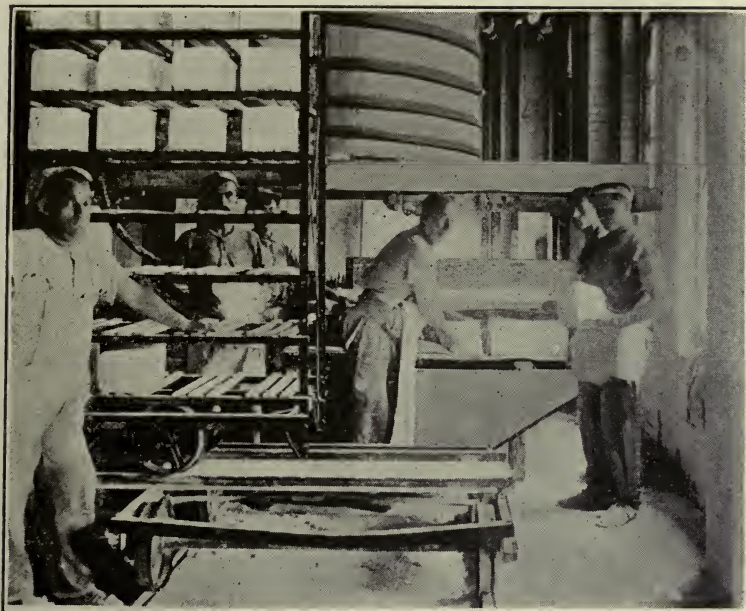
Fig. 31.—Emptying Starch from Drip Boxes. Breaking into Cubes. (Courtesy of Corn Products Refining Co.)
