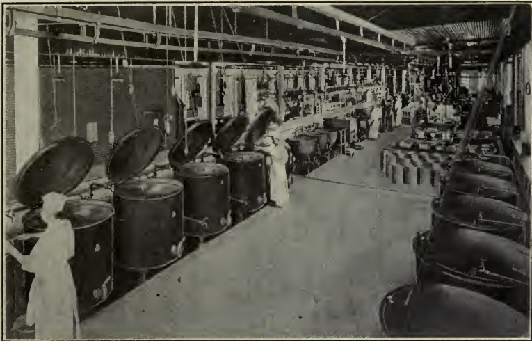
Fig. 62.—Stock Boilers. (Courtesy of the Franco-American Food Co.)
