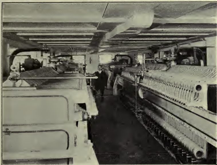
Fig. 45.—Filter Presses for Clarifying the Wort. (Courtesy of United States Brewers' Association.)
