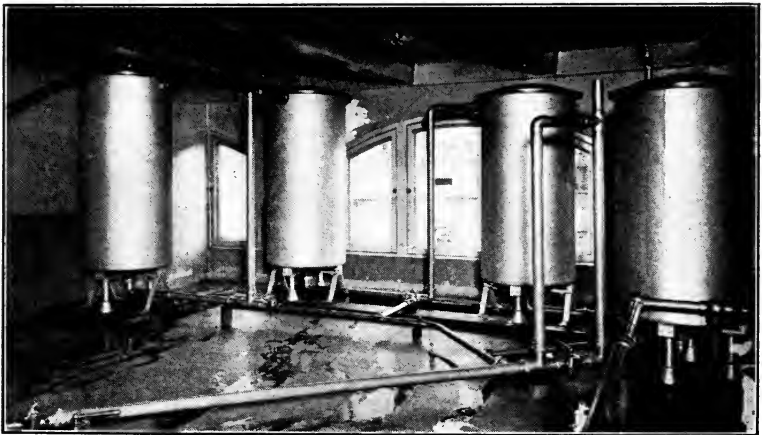
Fig. 57.—Holding Tanks. Milk heated to 145^{\circ} F. is conducted successively to four holding tanks where it is held for fifteen minutes in each tank. At a temperature of about 142^{\circ} F. it passes back through the pasteurizers and is rapidly cooled. (Courtesy of the Sheffield-Farms-Slawson-Decker Co.)
