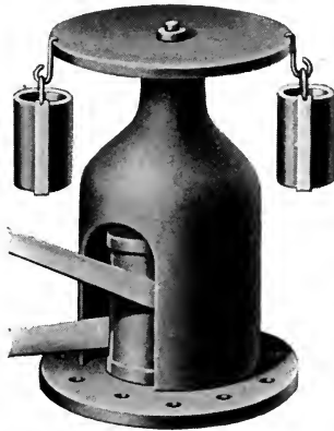
Fig. 48.—Early Experiment in Cream Separator. (Courtesy of the De Laval Cream Separator Co.)
