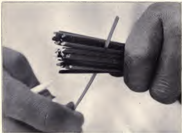
FIG. 2. STARTING THE COIL. END OF THREAD MATERIAL INSERTED BETWEEN STRANDS OF COIL.
