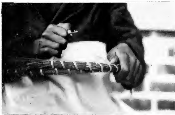
FIG. 23. STARTING TO BUILD UP THE SIDE OF THE BASKET.
