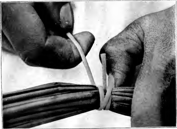
FIG. 6. STARTING THE COIL—THE TIE
