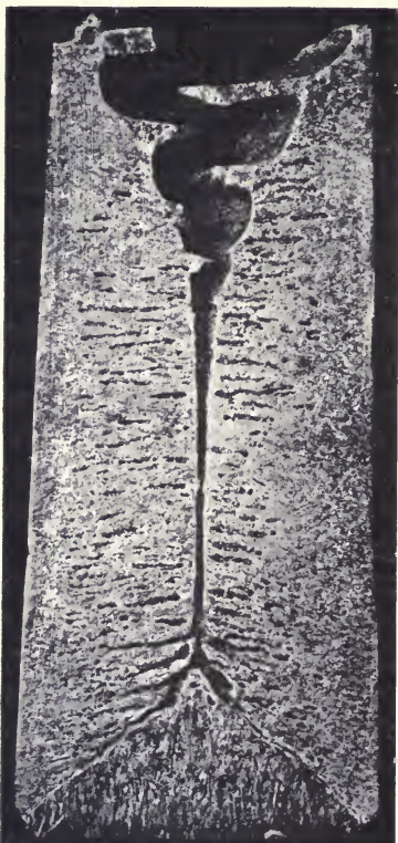
FIG. 12.—Diagonal contraction cavities.
