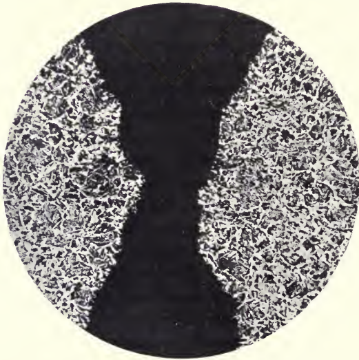
FIG. 41.—Structure of material about bright cavities \times 16 .
