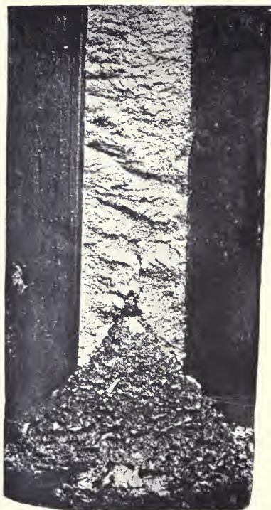
FIG. 4.—Exposed pyramid in base of steel ingot.
