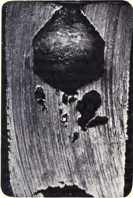
FIG. 50.—Section through head of inverted ingot.
