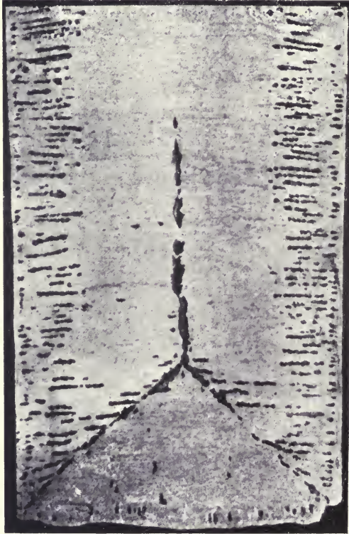
FIG. 99.—Ingot section, showing cavities on base pyramid.
