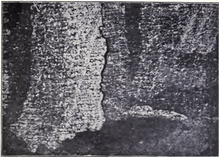
FIG. 14.—Fig. 1 enlarged to show crack between crystals.
