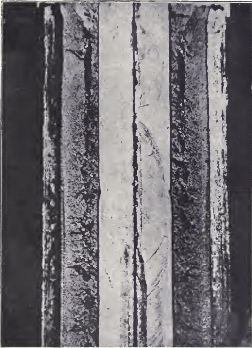
FIG. 31a.—Cavities below dozzle in crucible ingots.
