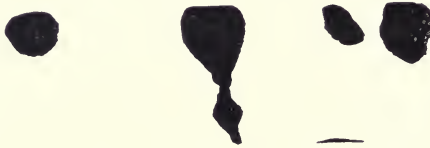
FIG. 40.—Gas cavities at base of large ingot.
