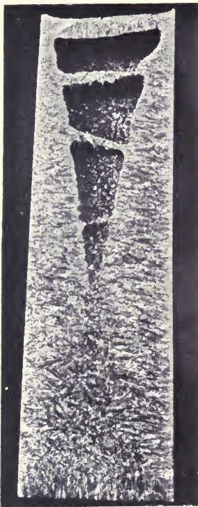
FIG. 53.—Deflected pipe due to unequal cooling.
