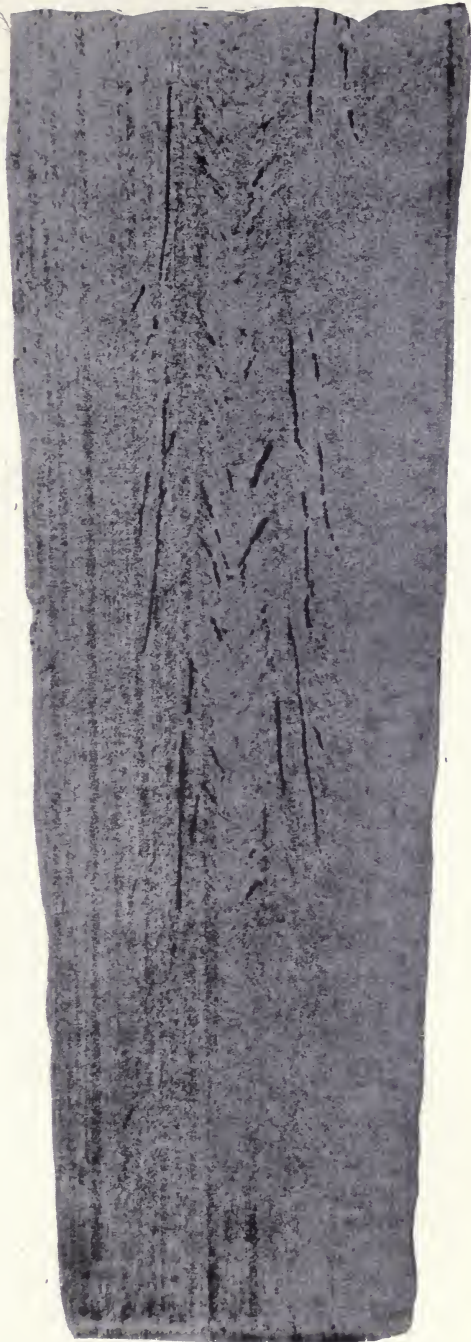
FIG. 81.—Sulphur print of large ingot, showing ghosts.
