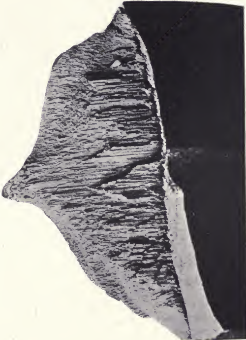
FIG. 101.—Fibre in spring steel bar.
