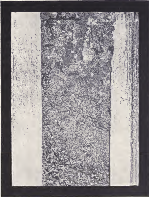
FIG. 56.—Carburizing effect of charcoal in dozzle.
