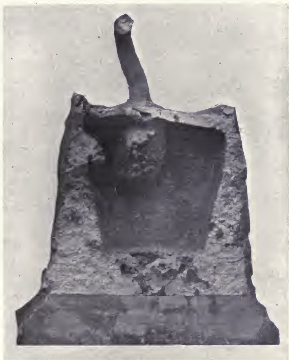
FIG. 70.—Split head to show effect of lifting hoops.
