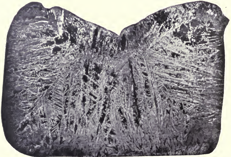
FIG. 84.—Crystalline growth in spoon-test sample.
