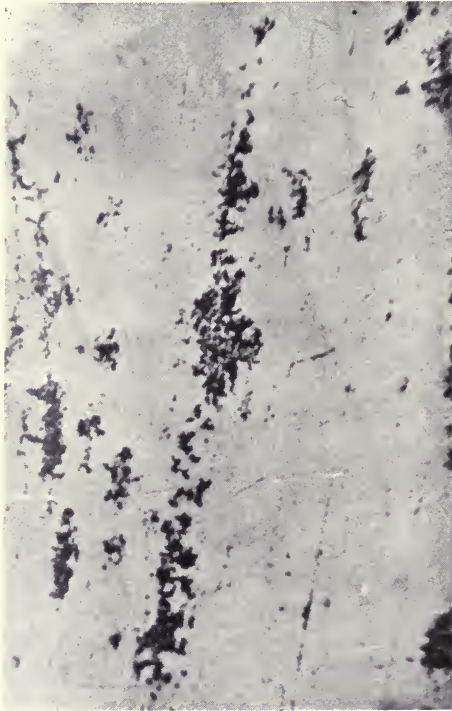
FIG. 88.—Aggregated alumina in cutlery steel \times 100 .
