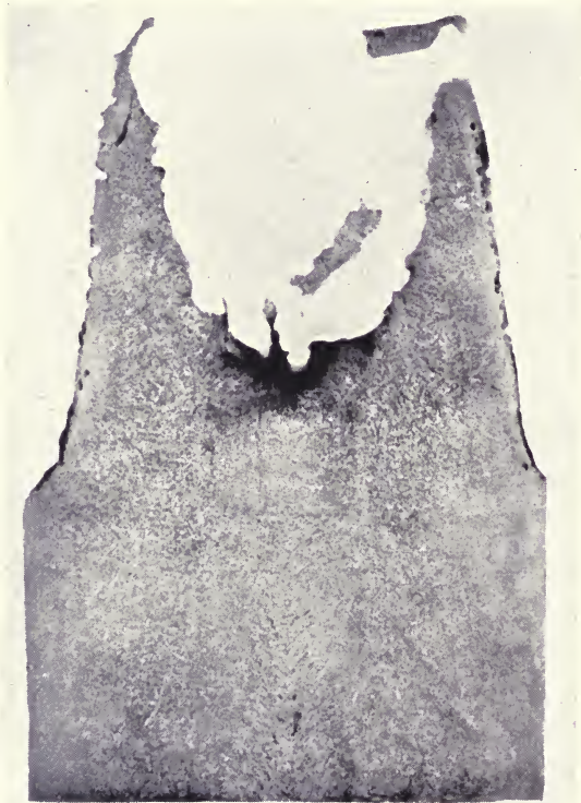
FIG. 69.—Sulphur print of ingot head.
