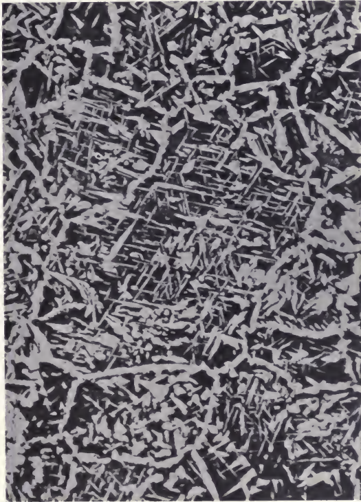
FIG. 63.—Re-heated ingot or billet structure \times 25 .
