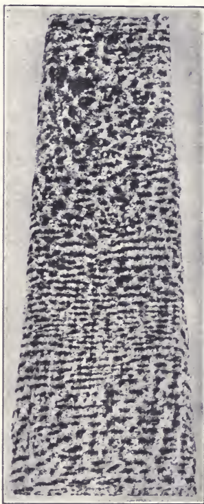
FIG. 18.—Appearance of surface of "cold cast" ingot.
