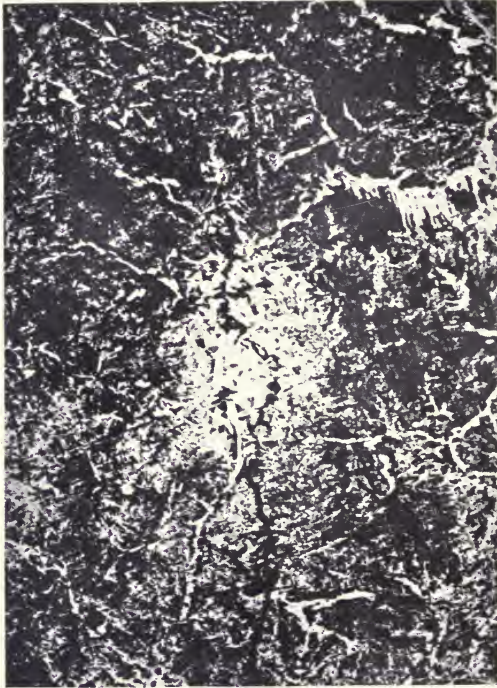
FIG. 16.—Radial crack in 30-ton steel billet.
