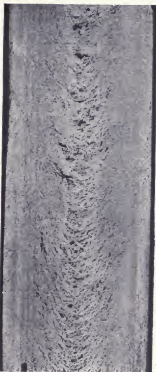
FIG. 54.—Shrinkage depressions in German silver ingot.
