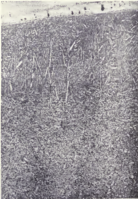
FIG. 73.—Sulphur print of top-poured ingot.
