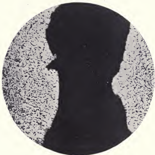
FIG. 42.—Structure of material about oxidized cavities \times 16 .
