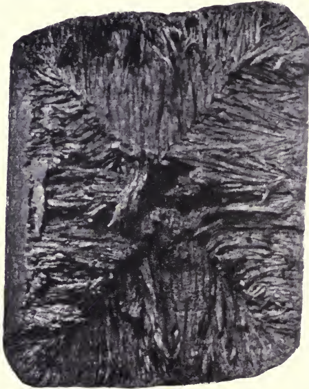
FIG. 26.—Fracture of "hot-cast" nickel steel ingot.
