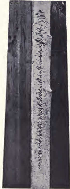
FIG. 61.—Shrinkage cavity in Harmet steel ingot.
