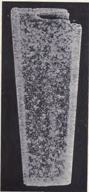
FIG. 21.—Deposited free crystals in solid wax ingot.
