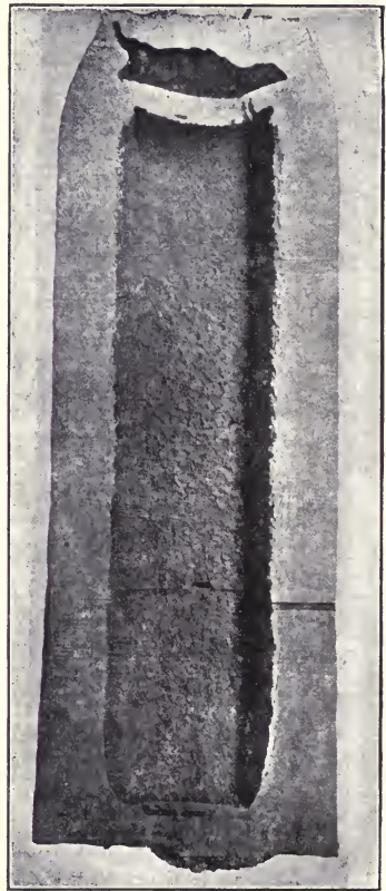
FIG. 11.—Open-hearth ingot intentionally bled.
