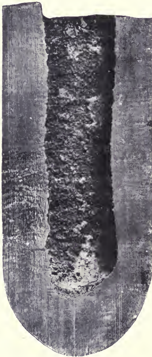
FIG. 10.—Partly fluid crucible ingot intentionally inverted.
