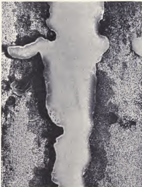
FIG. 83.—Sulphide segregation in pipe of ingot.
