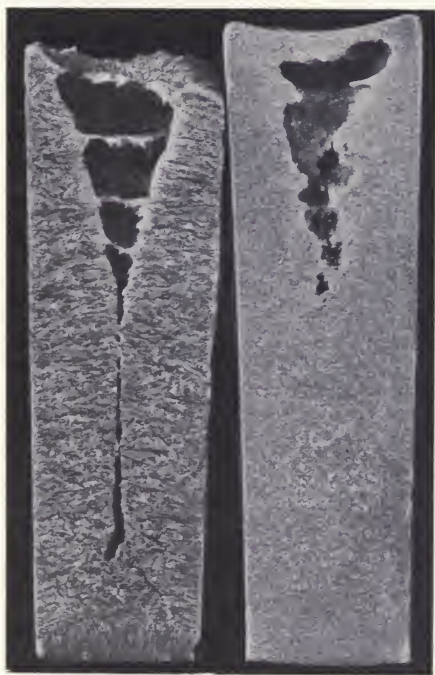
FIG. 33.—Relative shrinkage and contraction in hot- and cold-cast ingots.
