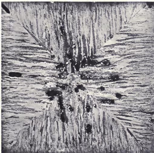
FIG. 15.—Cracked surfaces corroded by pickling.
