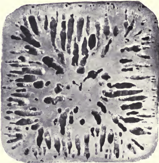
FIG. 75.—Blow-holes caused by rusty moulds.
