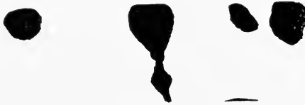
FIG. 40.—Gas cavities at base of large ingot.
