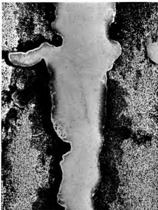
FIG. 83.—Sulphide segregation in pipe of ingot.
