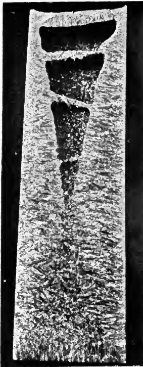
FIG. 53.—Deflected pipe due to unequal cooling.
