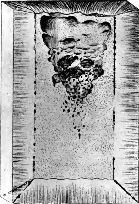
FIG. 37.—Planes of weakness in flat ingots.
