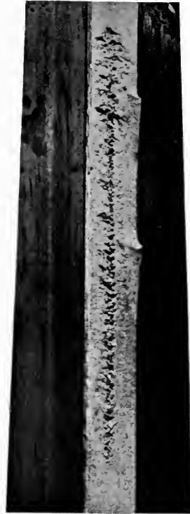
FIG. 61.—Shrinkage cavity in Harmet steel ingot.
