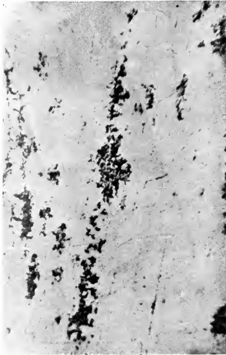
FIG. 88.—Aggregated alumina in cutlery steel \times 100 .
