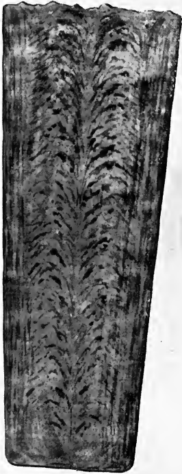
FIG. 66.—Section of sound ingot etched with Heyn's reagent.
