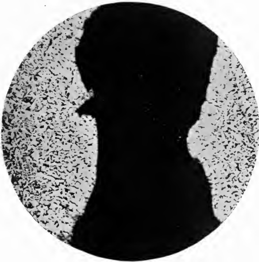
FIG. 42.—Structure of material about oxidized cavities \times 16 .
