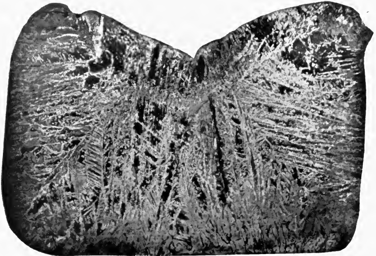
FIG. 84.—Crystalline growth in spoon-test sample.
