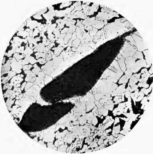
FIG. 93.—Ferrite envelope around slag enclosure.
