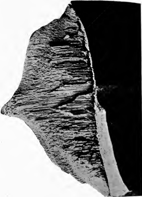
FIG. 101.—Fibre in spring steel bar.
