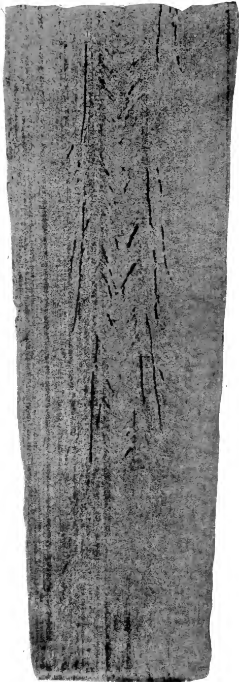
FIG. 81.—Sulphur print of large ingot, showing ghosts.
