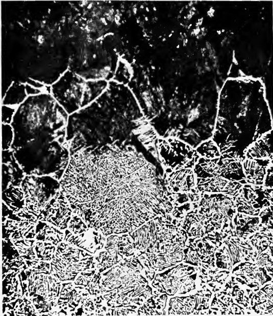
FIG. 77.—Inner edge of carburized envelope of mild steel.
