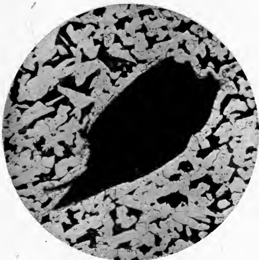
FIG. 94.—Ferrite envelope around silica sand.
