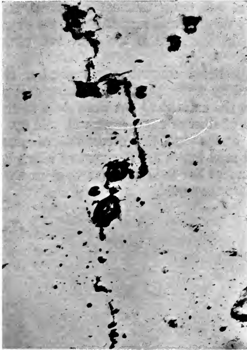
FIG. 17.—Easy passage of radial crack between slag occlusions.
