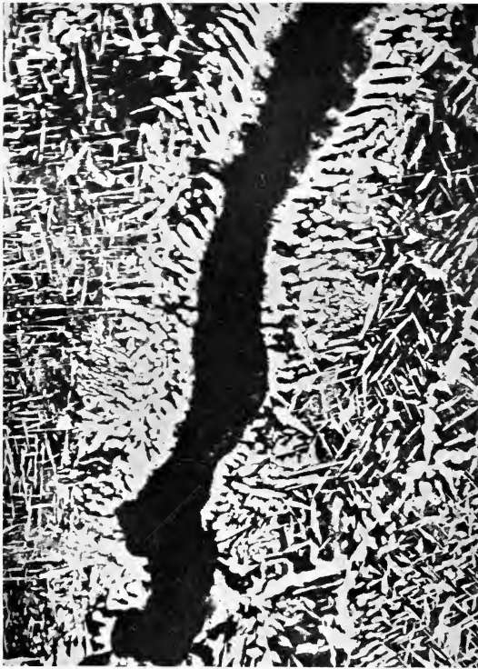
FIG. 13.—Rupture along diagonal plane of steel ingot. \times 25 .
