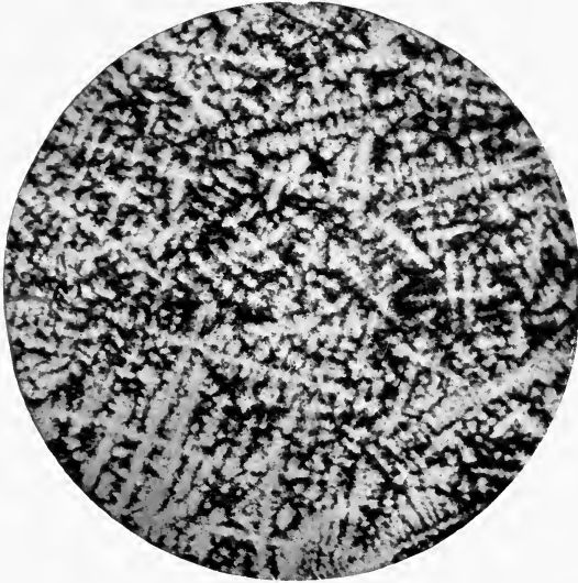
FIG. 91.—Dendrites in forged piston rod.
