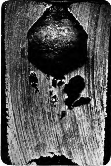
FIG. 50.—Section through head of inverted ingot.
