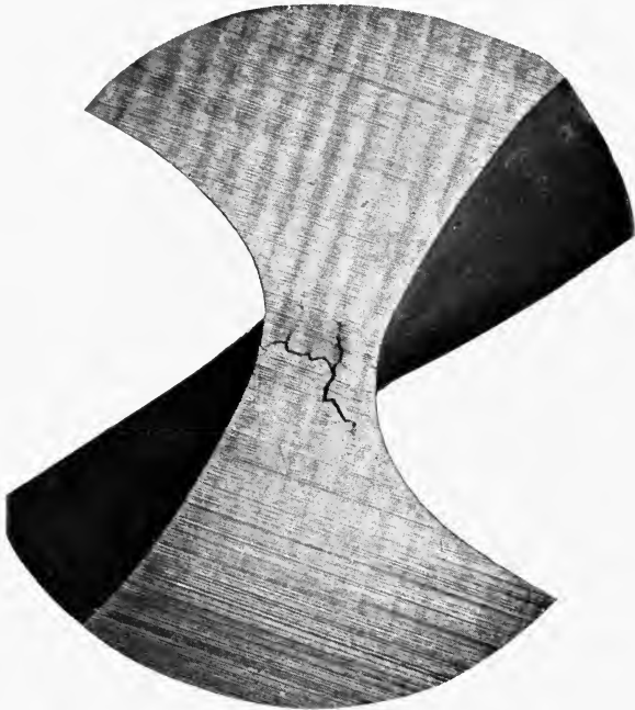
FIG. 55.—Cracked centre in bar steel arising from axial cavity in ingot.
