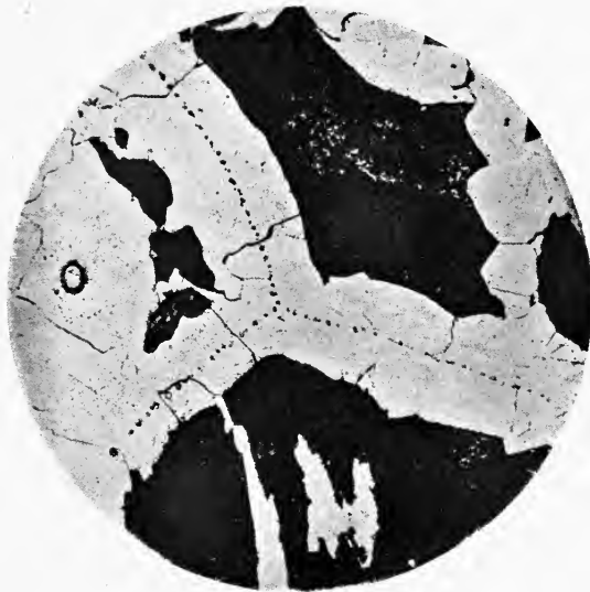
FIG. 89.—Slag particles between primary crystals.
