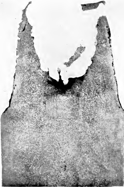
FIG. 69.—Sulphur print of ingot head.
