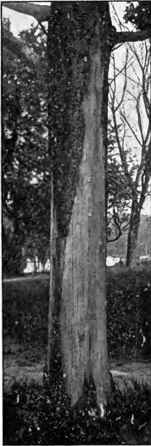
Fig. 7. Maple tree killed by direct current from a trolley system, carrying positive current through the rail, and return current through the feed wire in contact with branches. The largest amount of burning occurred slightly remote from the point opposite the rail, and in line with a large root, lying diagonally with, and just under the nearest rail.
