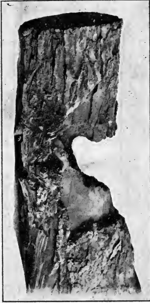
Fig. 5. Showing deep burning of a large limb, caused by an alternating wire of high potential. From Luke Doogue, City Forestry Dept., Boston.
