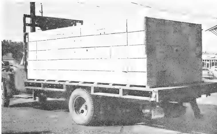
Figure 26.--Tie cable with corner plates to secure load on a road truck bed.
