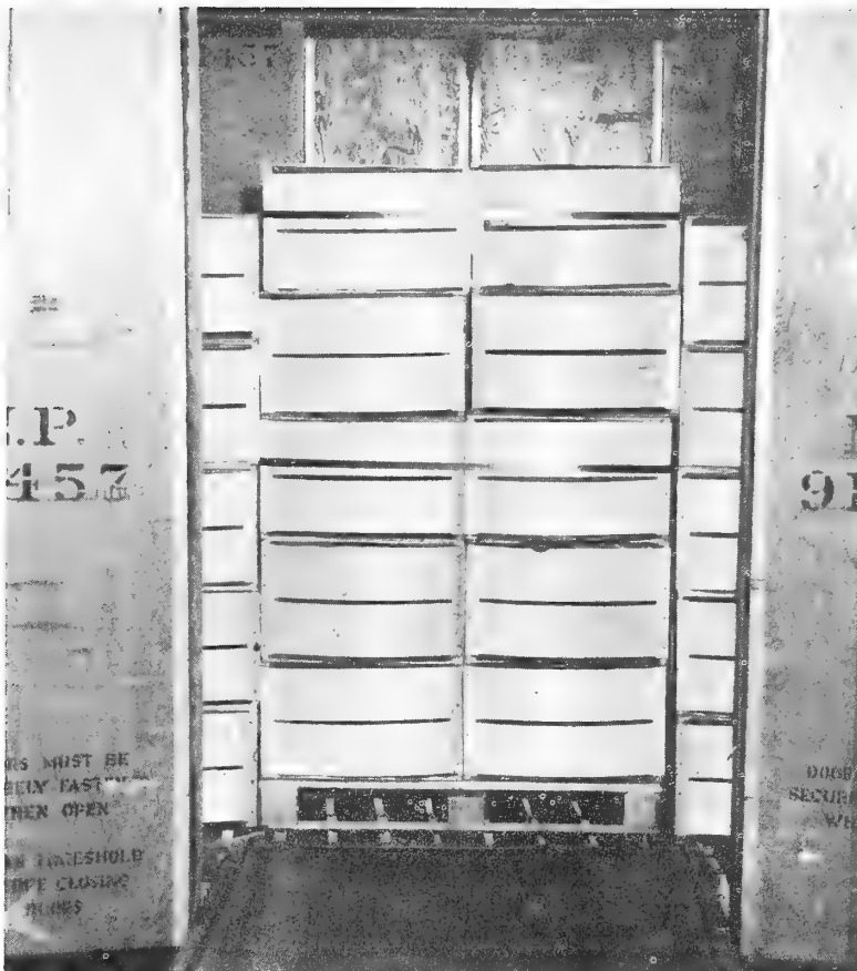
Figure 37.--Loading the doorway of a refrigerator car when boxes are partially palletized.
