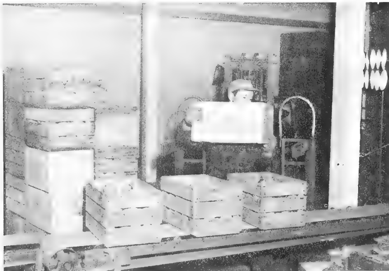
Figure 19.--Operator of an industrial clamp-type lift truck placing boxes on the belt conveyor.
