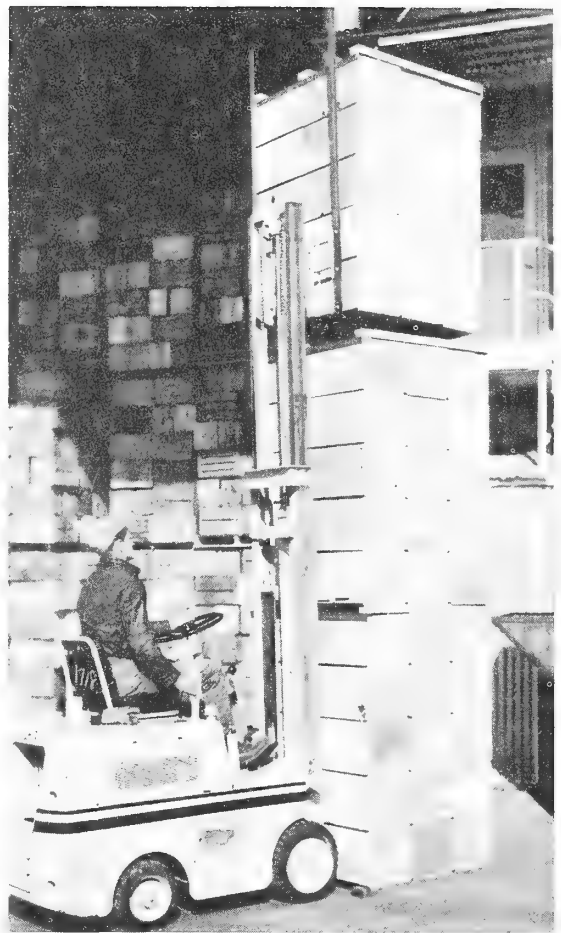
Figure 30.--Release of third tier of boxes by broad-blade forklift truck. Top tie frame on second tier allows fork to be retracted.
