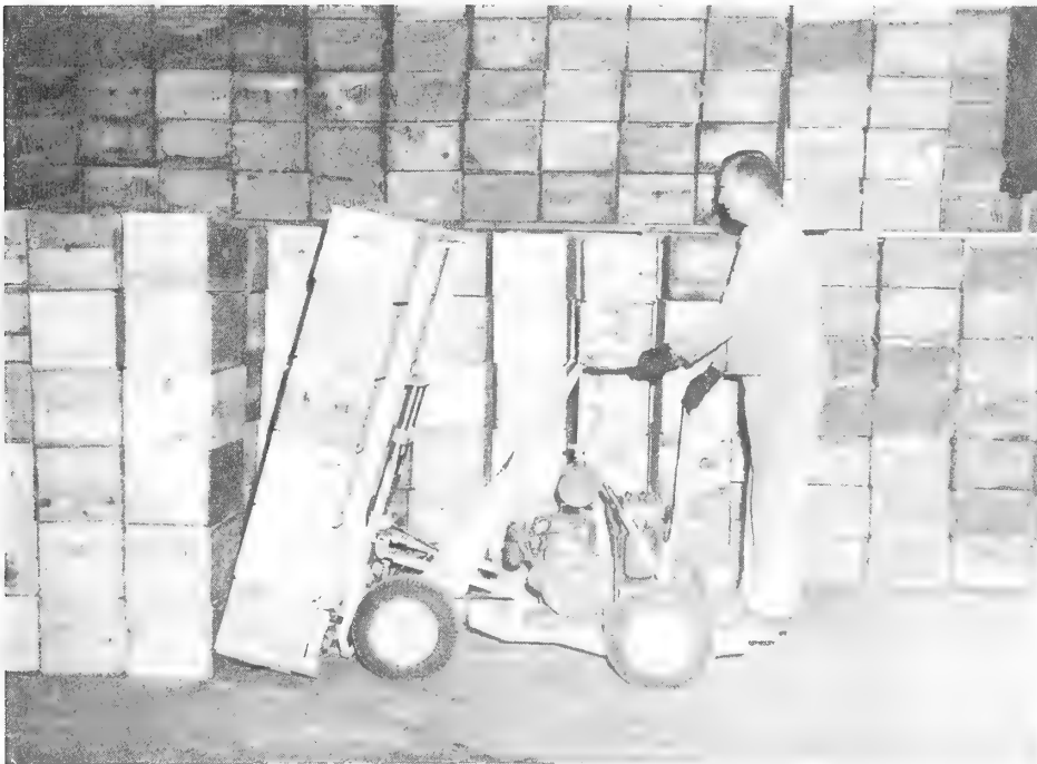
Figure 22.--Moving stacks of boxes from storage to the packing line with a 12-box industrial clamp-type truck.
