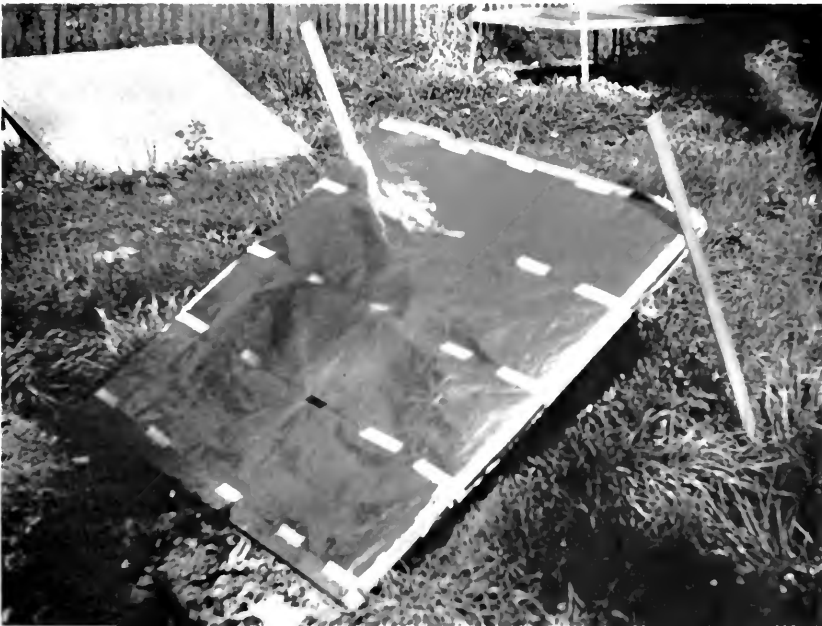
This reflector shield is about 4 feet square, made of hardboard and framed with pine strips; the under (reflecting) side is covered with household-type aluminum foil fastened with pressure-sensitive paper tape. The supporting stakes should have been heavier. The shields were kept as close to the stump as practical, as shown by those in the background. (Fig. 2)
