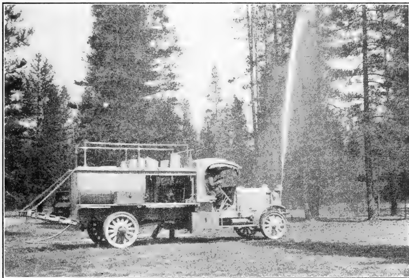
FIGURE 84.—High-pressure spraying outfit used along highways of the Shoshone National Forest, Wyo.
