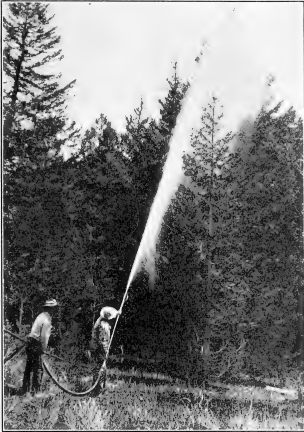
FIGURE 85.—A long hose permits reaching out for distances of 1,500 to 5,000 feet from the spray pump.
