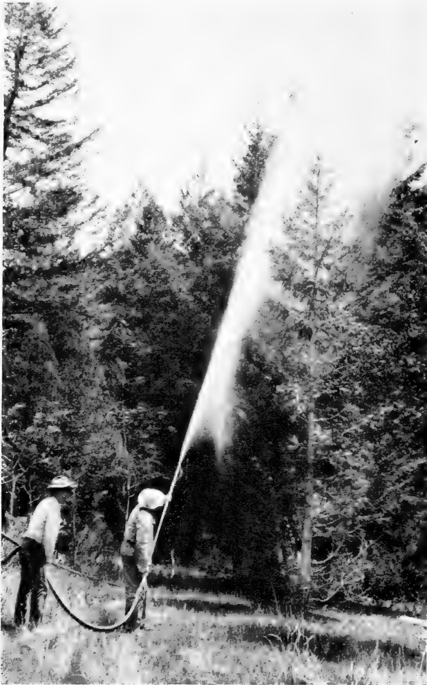
FIGURE 103.—With a long hose it is possible to reach distances of 1,500 to 5,000 feet from the spray pump.
