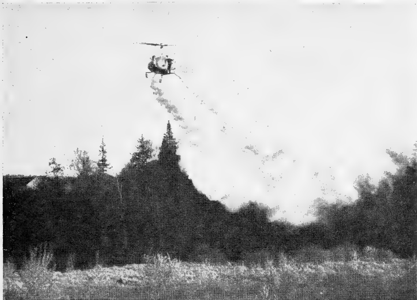
FIGURE 21.—Helicopter with thermal smoke generator in operation.
