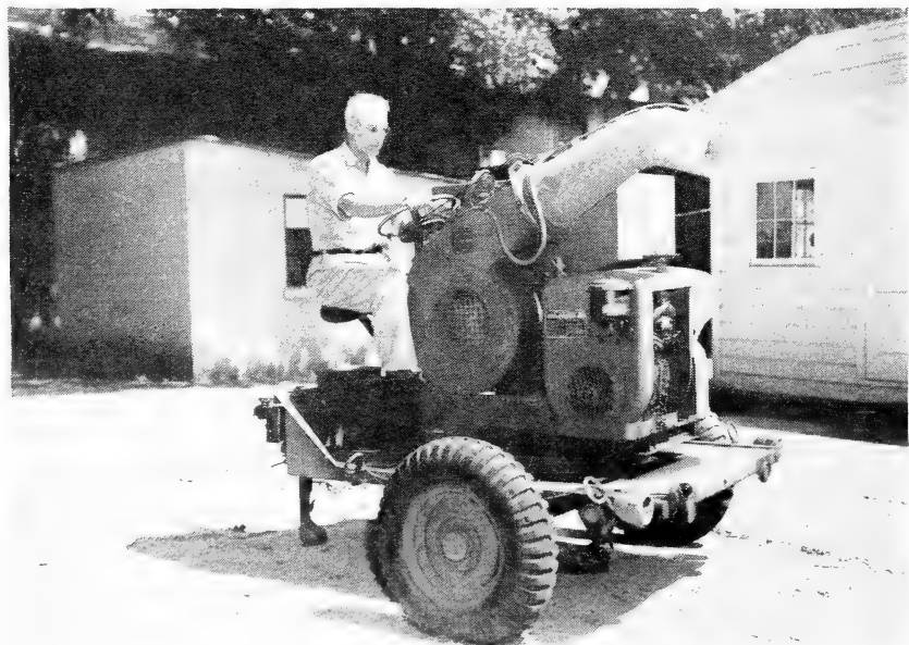
FIGURE 8.—One type of mist blower used experimentally by Army engineers.
