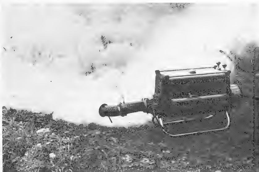
FIGURE 12.—Jet-type fog machine in operation.
