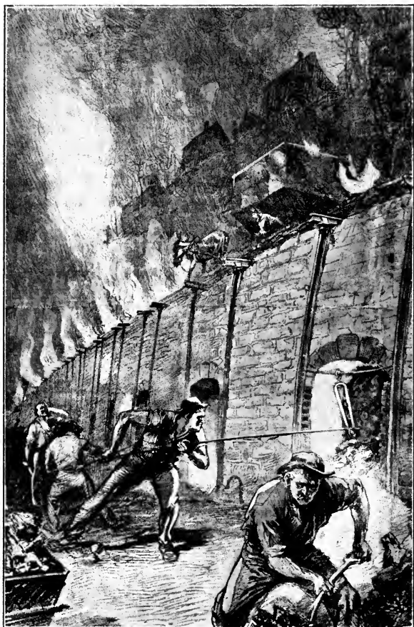
Drawing the finished coke. The method of charging the raw coal is also seen. It is dropped from the donkey-car through an opening in the top of the oven.
