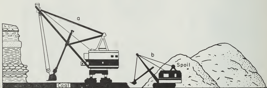
Figure 11 - Diagram of strip mine showing: (a) stripping shovel, and (b) coal-loading shovel.
