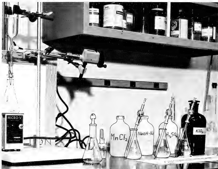
Figure J-4. (Micro) Winkler apparatus.
