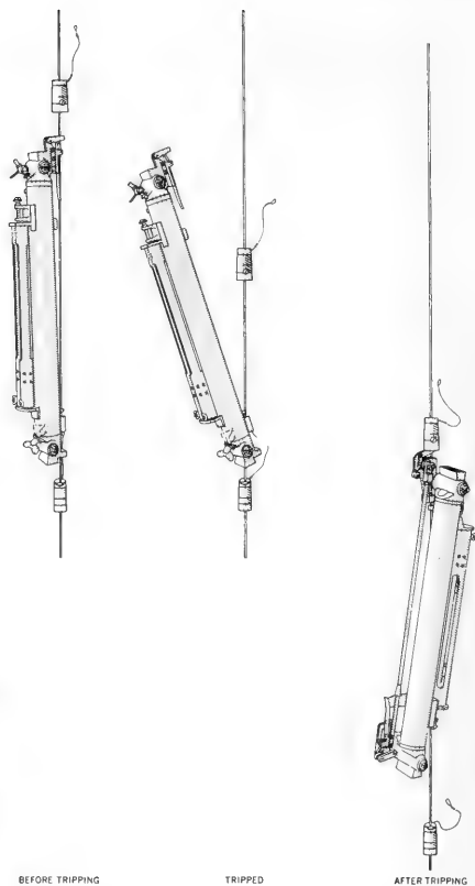
Figure D-4. Nansen bottle in three positions—before tripping, during tripping, and after tripping.
