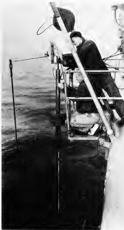
Figure L-6. Taping bight of lowering wire to Kullenberg corer.
