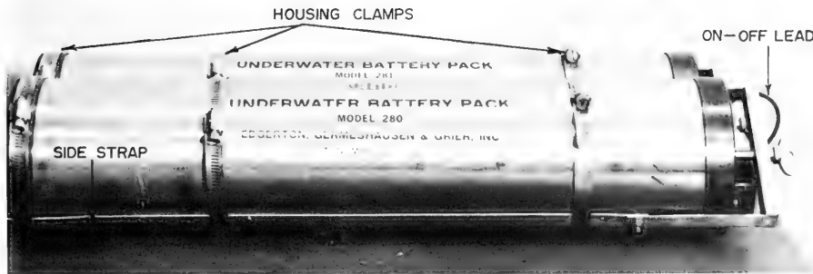
Figure N-4. Underwater battery packs (Model 280 contains time delay unit and Model 281 contains 15-second cycling device).
