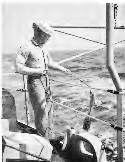
Figure 2-12. Bringing in the BT with a retrieving line.
