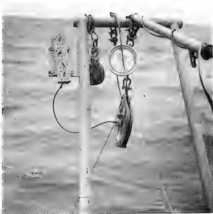
Figure L-15. Dynamometer attached to retractable A-Frame.
