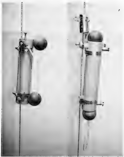
Figure O-12. Frautschy water sampling bottle before and after tripping.
