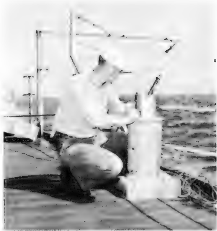
Figure C-9. Reading the sea surface reference temperature.
