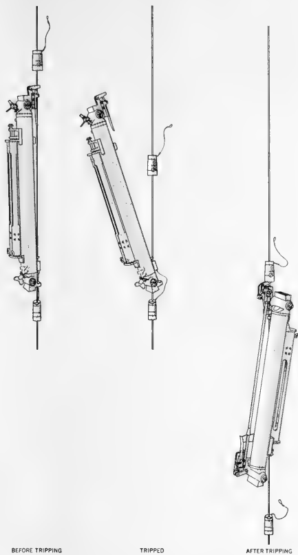
Figure 2-1. Nansen bottle in three positions—before tripping, during tripping, and after tripping.
