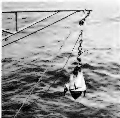
Figure L-17. Orange Peel bucket sampler rigged for lowering.
