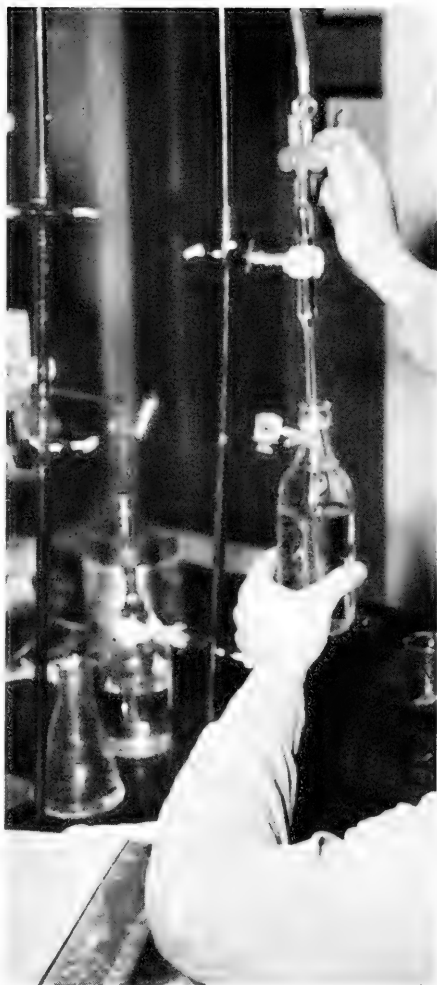
Figure 13-3. Drawing the salinity sample with the pipette.
