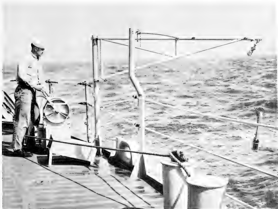
Figure 2-11. Lowering the bathythermograph.
