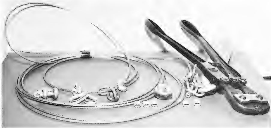
Figure C-5. The Nicopress tool and sleeves, wire rope, thimbles, swivels, wire clips, and shackles.
