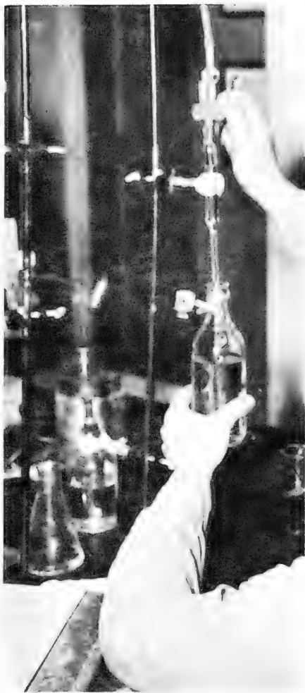
Figure I-5. Drawing the sample with the automatic pipette.
