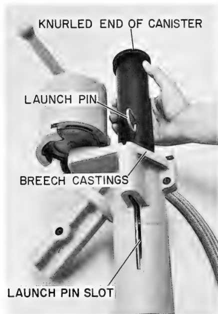
Figure C-22. Loading canister in breech.
