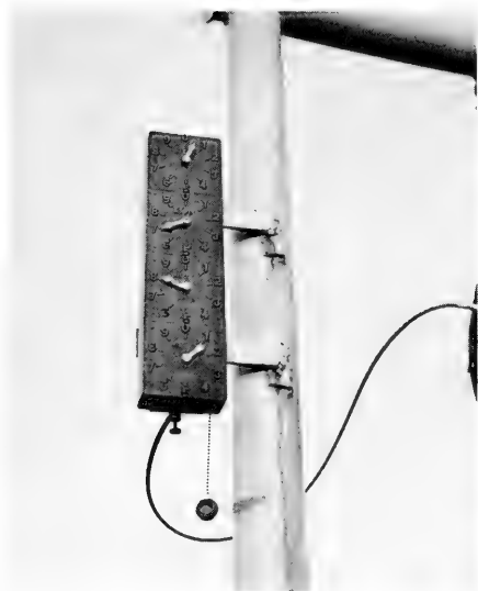
Figure 2-3. A meter wheel reading of a Nansen bottle cast.
