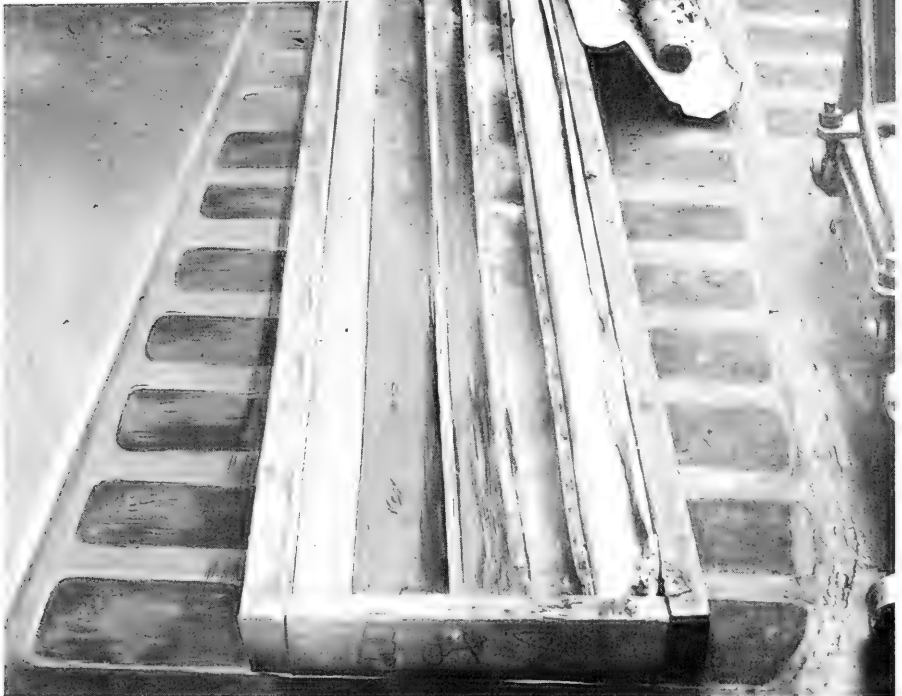
Figure 6-10. Extruding and packing Ewing cores.
