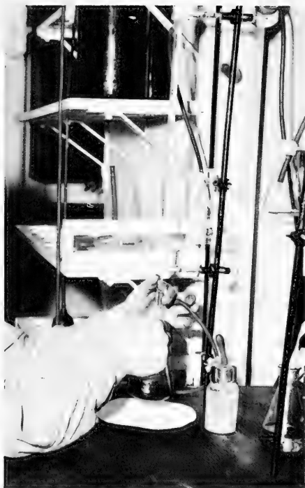
Figure 13-9. Titrating the dissolved oxygen sample.
