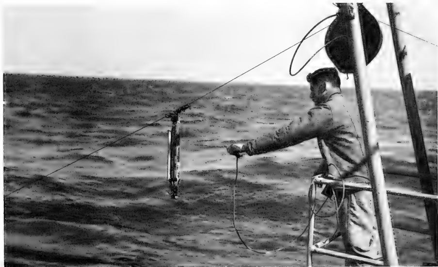
Figure E-7. Snapping the safety line onto the bottle.
