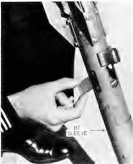
Figure C-7. Inserting glass slide into BT.
