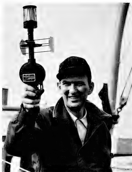
Figure B-27. Measuring wind speed and direction with Wind Measuring Set (AN-PMQ-5A).
