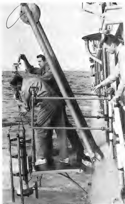
Figure R-1. Sonar pinger replaces weight on Nansen cast.
