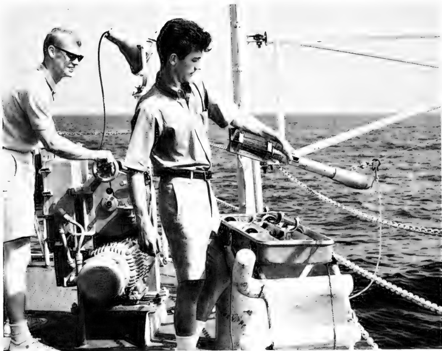
Figure C-10. Bringing BT aboard with a retrieving line and ring.
