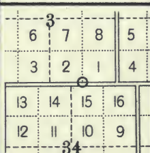
Fig. 22. Corner of L. S. 3, 4, 5 and 6 of sec. 23. Legal subdivision corner in the interior of a section.
