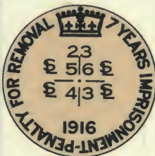
Fig. 22. Corner of L. S. 3, 4, 5 and 6 of sec. 23. Legal subdivision corner in the interior of a section.
