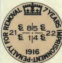
Fig. 24. Corner of L. S. 4 and 5 of sec. 22 and L. S. 1 and 8 of sec. 21. Legal subdivision corner on meridian section line.
