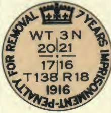
Fig. 9. N.E. corner 17-138-18 Witness to section corner in interior of township.
