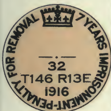
Fig. 20. \frac{1}{4} sec. cor. on North By. 32-146-13 E. Quarter sec. cor. south of correction line.
