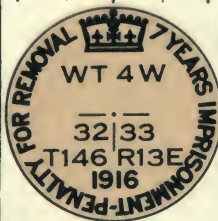
Fig. 14. N.E. cor. 32-146-13 E Witness to section cor. south of correction line
