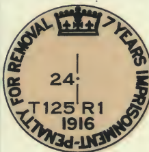
Fig. 21. \frac{1}{4} sec. cor. on East By. 24-125-1 Quarter sec. cor. on initial meridian.
