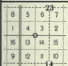
Fig. 20. \frac{1}{4} sec. cor. on North By. 32-146-13 E. Quarter sec. cor. south of correction line.
