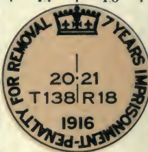
Fig. 16. \frac{1}{4} sec. cor. between 20 and 21-138-18 Quarter sec. cor. in interior of township.
