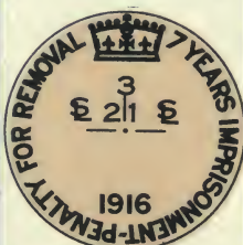
Fig. 25. Corner of L. S. 1 and 2 of sec. 3. Legal subdivision corner on correction line.
