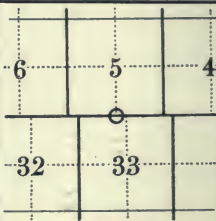
Fig. 16. \frac{1}{4} sec. cor. between 20 and 21-138-18 Quarter sec. cor. in interior of township.
