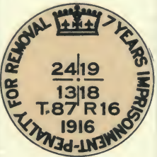
Fig. 11. N.E. corner 13-87-16 Section corner on east outline of township.
