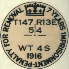
Fig. 13. S.E. corner 5-147-13E Witness to section corner on north side of correction line.
