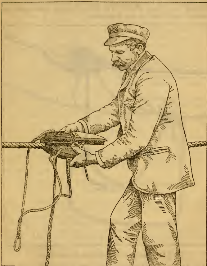
FIG. 16.—Applying hawser cutter.
