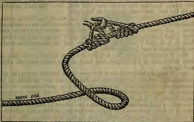
FIG. 11.—Manner of adjusting strap to hawser.
