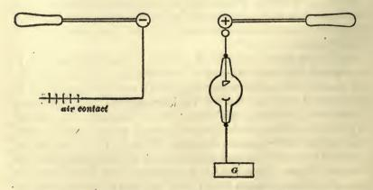
One of these arrangements is represented in the annexed figure, where the cathode terminal of the tube is grounded on the gas-pipe,
