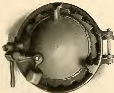
Bottom of hopper showing cut-off, seed plate and agitating ring
