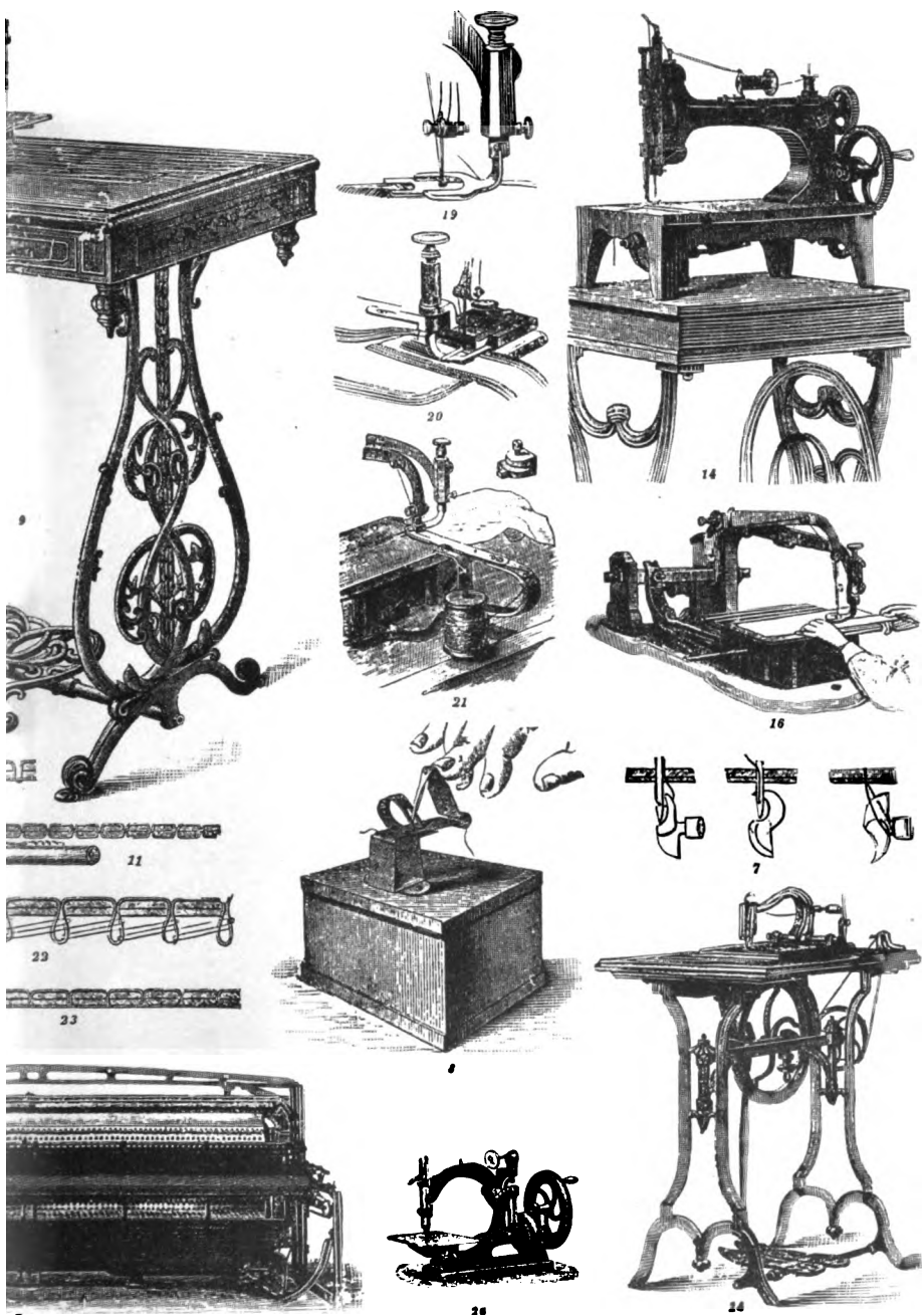
6. Single-thread chain-stitch; 7, formation thereof. 8. Heyer's (simplest form of) sewing machine and back stitch (or quilt-stitch); 12, its formation on bobbin machines. 13. "No-tension" treadle-less machine. 17, 18. Formation of stitches by Wheeler & Wilson machines. 19. Presser foot of treadle-less sewing machine. 25. Shoemakers' sewing machine. 26. Automatic hand-machine.
