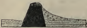
FIG. 25.—Diagrammatic section of an old volcanic neck forming a crag, with a "tail" of boulder clay.
