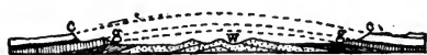
FIG. 84.—Section across the Weald from North to South. cc Chalk, gs Greensand escarpments, w Wealden sandstones
