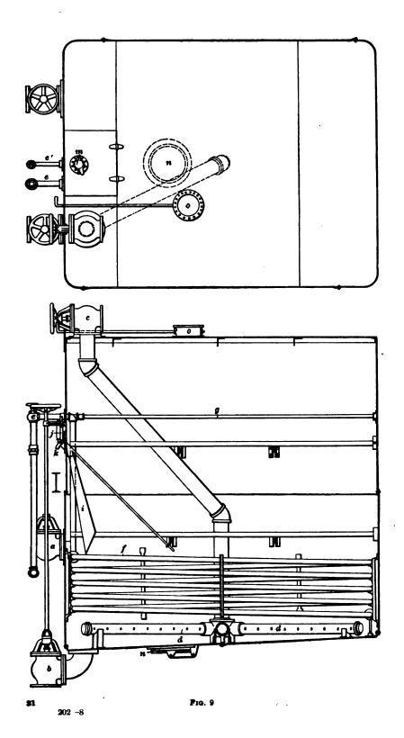
The carbonatation and saturation may also be conducted in a continuous carbonator; that is, an apparatus into which limed juice is constantly flowing and from which there is a continuous stream of carbonated juice. Such apparatus, however, is seldom used.
