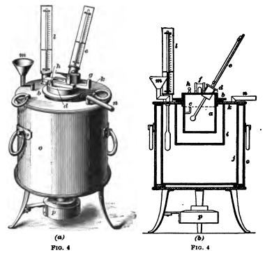
tilted in such an angle as to bring the end of the spout just below the surface of the lid. Upon the slide being pushed back so as to cover the holes, the lamp returns to its original position. Upon the cover, in front of, and in line with, the mouth of the lamp, is fixed a white bead h, the dimensions of which represent the size of the test flame to be used. The bath, or heated vessel, consists of two flat-bottomed copper cylinders, an inner one i, 3 inches in diameter and
