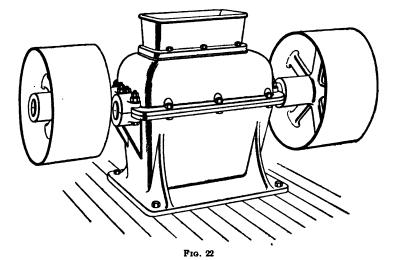
to prevent the cakes from souring and molding. After remaining until cool, which requires from 12 to 24 hours, the cakes are fed into a machine known as a cake breaker.
