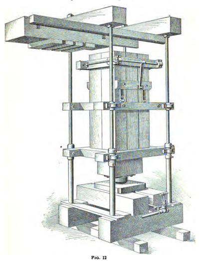
which is a convenient size for transportation. The loose hulls are compressed into bales by means of a hull packer, Fig. 12, which is similar in shape to a cotton-baling press
