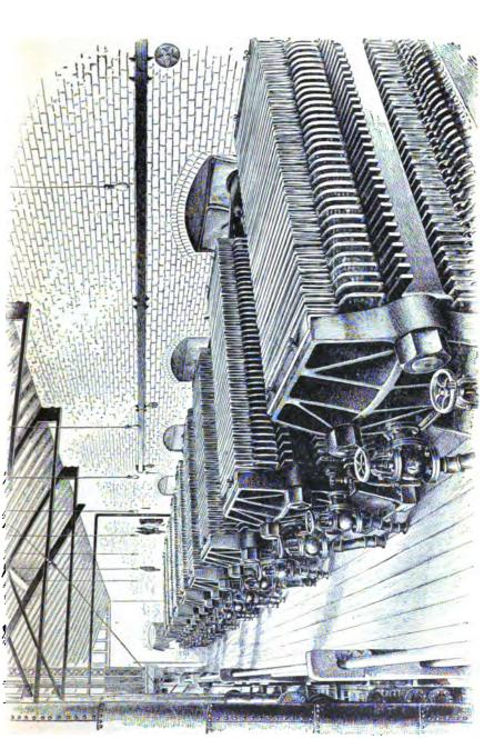
fills the spaces behind the cloths, passes into the press cake, and drives the juice ahead of it and through the open juice cocks to the trough. The frame presses often are designed to produce a cake about  $1\frac{1}{4}$  inches in thickness.
