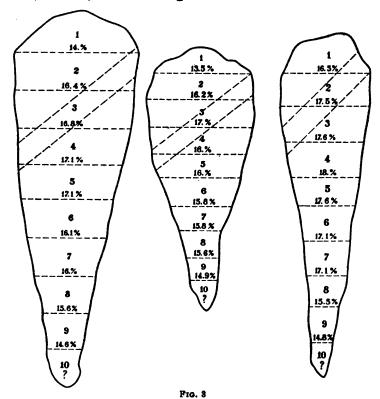
facture of Sugar, Part 1. Raffinose is present in small quantities and accumulates in the molasses. This sugar forms needle-shaped crystals and is not injurious in the manufacture. The distribution of the sugar in the beet, according to Slassky (Bul. Assoc. des Chimistes de France, 12, 277), is shown in Fig. 3.
