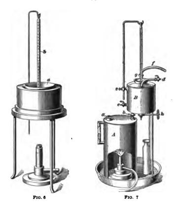
(see Quantitative Analysis). A great variety of these have been constructed, all based upon the length of time required for a given quantity of oil to flow through a small orifice, as compared with water or some other oil used as a basis. The best-known instruments are those of Saybolt, Tagliabue, and Engler.
