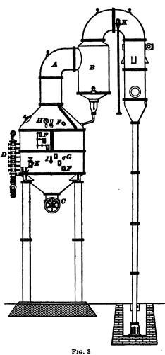
The degree of exhaustion of the pan, or, to use the usual sugar-house expression, the *vacuum*, is increased or decreased by increasing or decreasing the quantity of water injected
