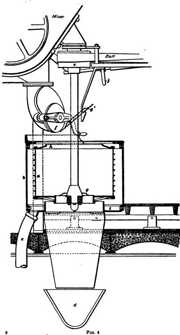
and to promote the development of the latter. The vapor pipe c connects the crystallizer with the vacuum pump through a condenser. It is claimed that crystallization is accomplished more quickly in a vacuum-pan crystallizer of this type than in the ordinary vacuum pan supplemented by crystallization in motion.
