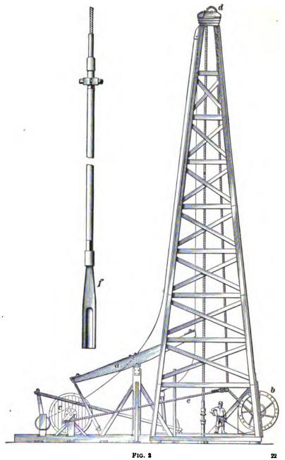
which it will be necessary to drill. In shallow-well territory, a shorter rig will materially reduce the cost of operation. Connected with the rig is a long, shed-like structure, known as the *belt house* and *engine house*. This contains the engine and band wheel c, which communicates its motion through a pitman with the walking beam a.
