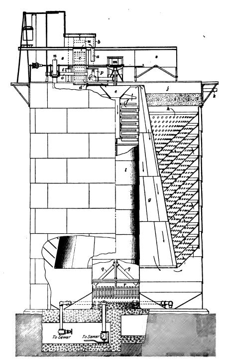
Railroad Company, and is extensively used by that railroad for softening water for locomotive use. This apparatus combines the features of the intermittent and continuous types. It has two settling tanks, which are alternately filled and emptied after the sludge has settled. The method of adding the softening solution, however, is continuous, and as this is the novel feature of the system, it is generally classed as a continuous apparatus.
