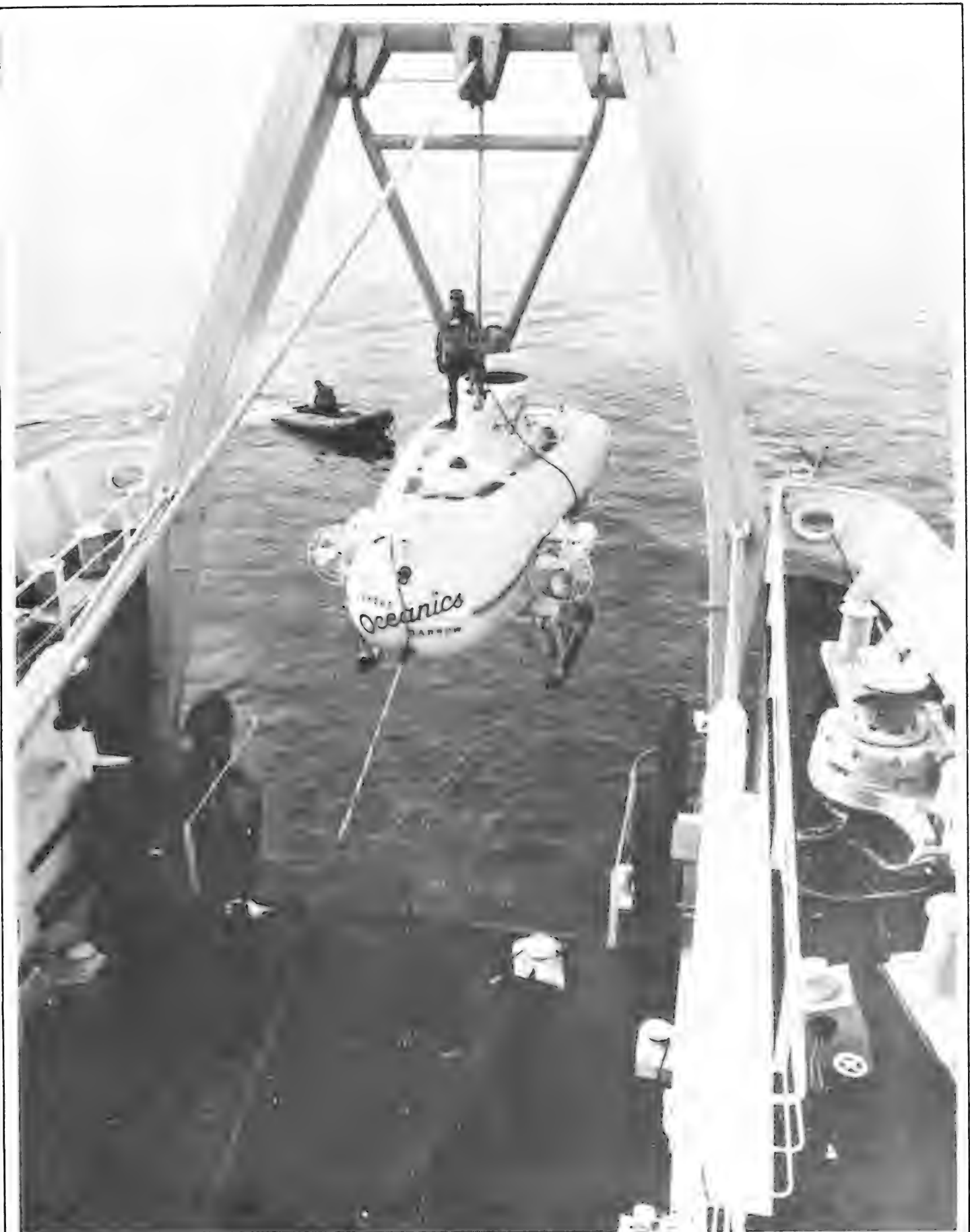
Fig.11. Vickers Oceanics Inc. Ltd.'s Support Ship and A-Frame Crane Handling PISCES III.
