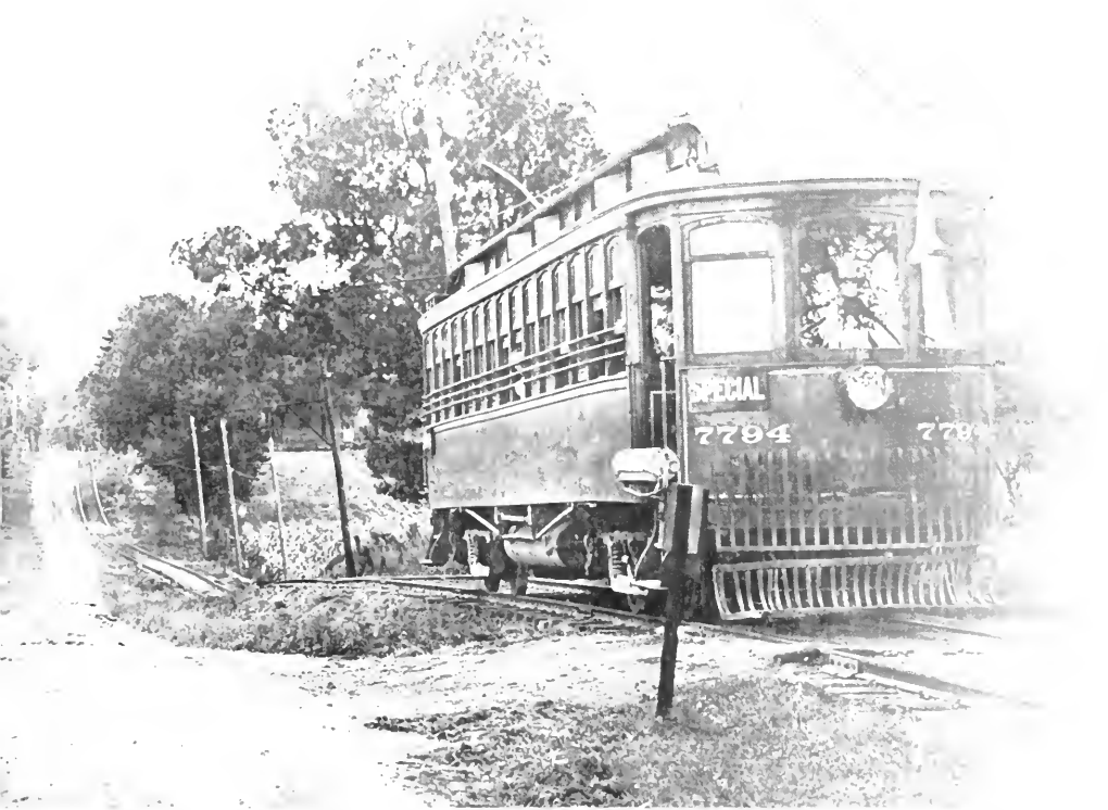
Detroit United car 7794 made a special trip over branch-line trackage which was an extreme example of the meandering, bill-and-dale, roadside variety of interurban construction. BARNEY NEUBERGER COLLECTION.
