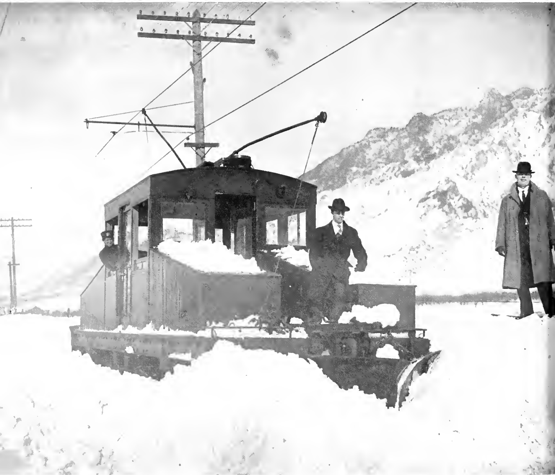
Winters were severe on the Utah interurbans, and scenes such as this were common. Home-built wooden freight locomotive No. 6 battled heavy drifts on the Ogden Rapid Transit line near Nerva before 1912. FRED FELLOW COLLECTION.
