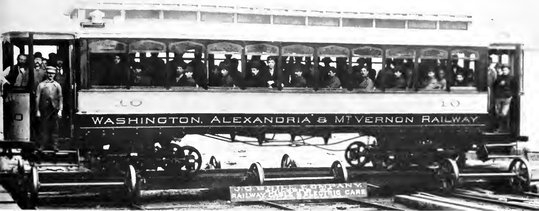
The distinctive architecture of the interurban car had not yet been evolved when J. G. Brill delivered this deck roof car for service on the Washington, Alexandria & Mt. Vernon Railway's new line to Alexandria in 1896. Nevertheless, the car was equipped with such interurban features as train doors for passage between cars, a lavatory, and a water cooler. It was capable of hauling one or two trailers at speeds up to 45 miles per hour. This carload of four individuals, probably Brill factory workers, simulated passengers for an advertisement that appeared in the February 1896 Street Railway Journal. LEROY O. KING COLLECTION.
