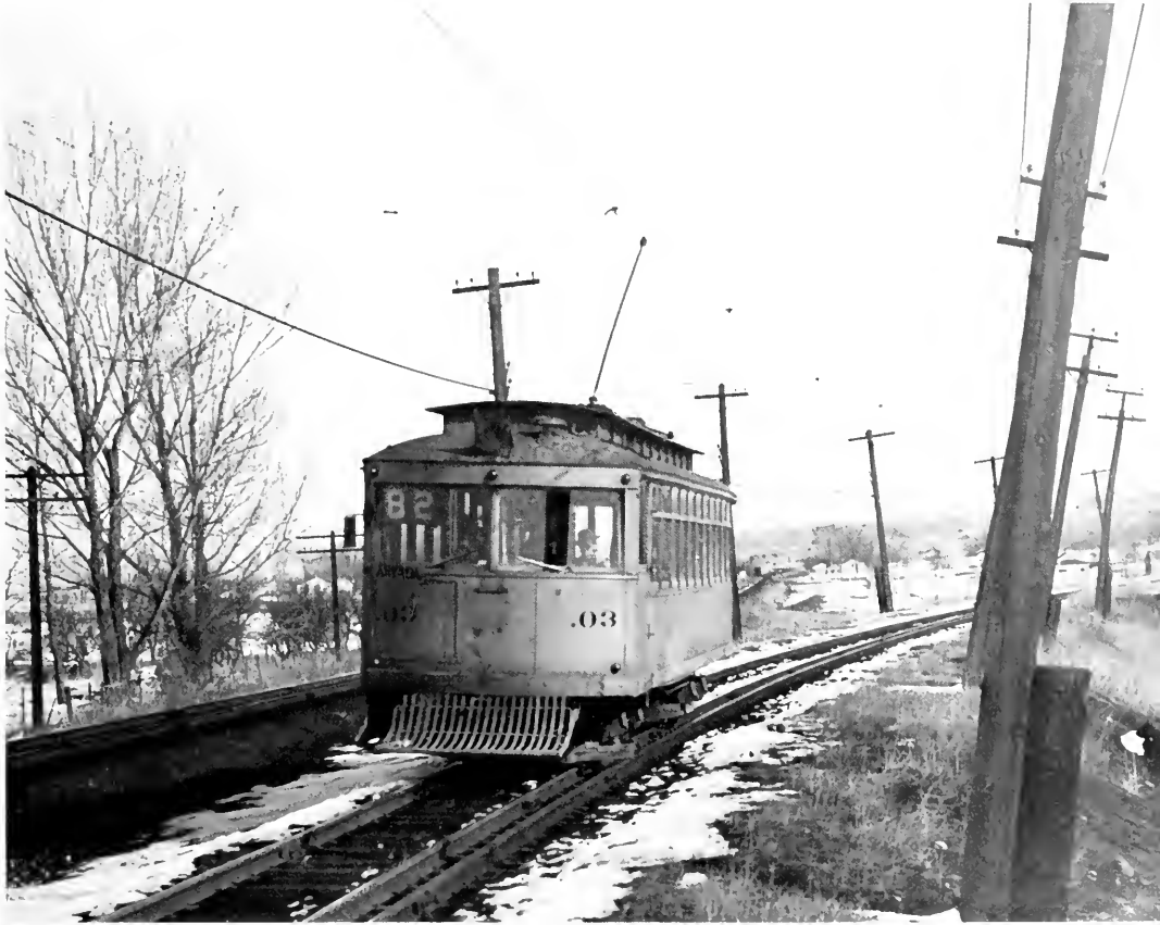
This D&IM narrow-gauge interurban, a converted city car, was running at a respectable 30 miles per hour near Arvada, Colo., in 1948 on dual-gauge track of the old Denver & Northwestern, which was parallel to the rails of D&RGW's Moffat-built transcontinental. A onetime funeral
