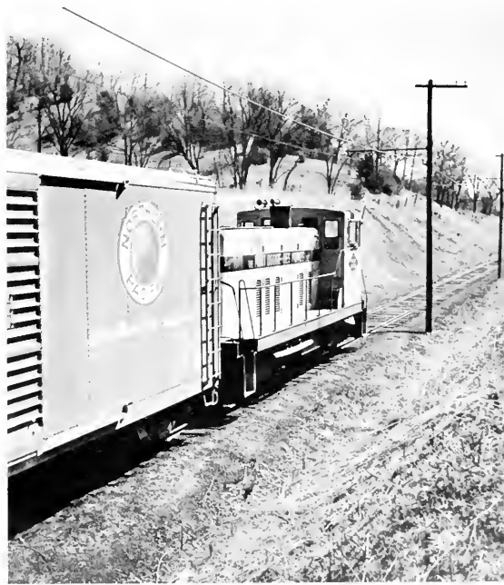
Almost all of the interurbans that have survived as freight-only carriers have abandoned electric equipment in favor of diesel-electric motive power. Iowa's Fort Dodge-Des Moines Line still employed both forms of power when this 70-ton General Electric diesel worked in the Des Moines River valley in 1955, but the railway has since taken down its trolley wire.
