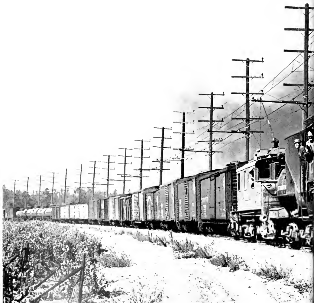
The extraordinary freight traffic of World War II was responsible for such dramatic activity as this combination of Mogul and steeple-cab working an eastbound extra freight through the vineyards near Etiwanda on the San Bernardino line. Overburdened with
