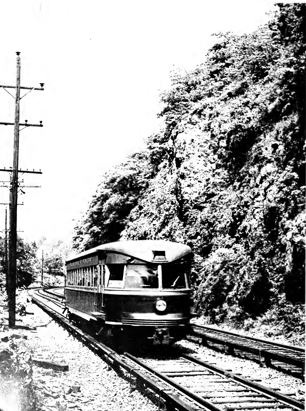
One of Dr. Conway's wind-tunnel-designed Bullet cars raced through Gulph Cut on the third-rail "super-interurban" Philadelphia & Western line, since 1954 a part of the Philadelphia Suburban system. WILLIAM D. MIDDLETON.
