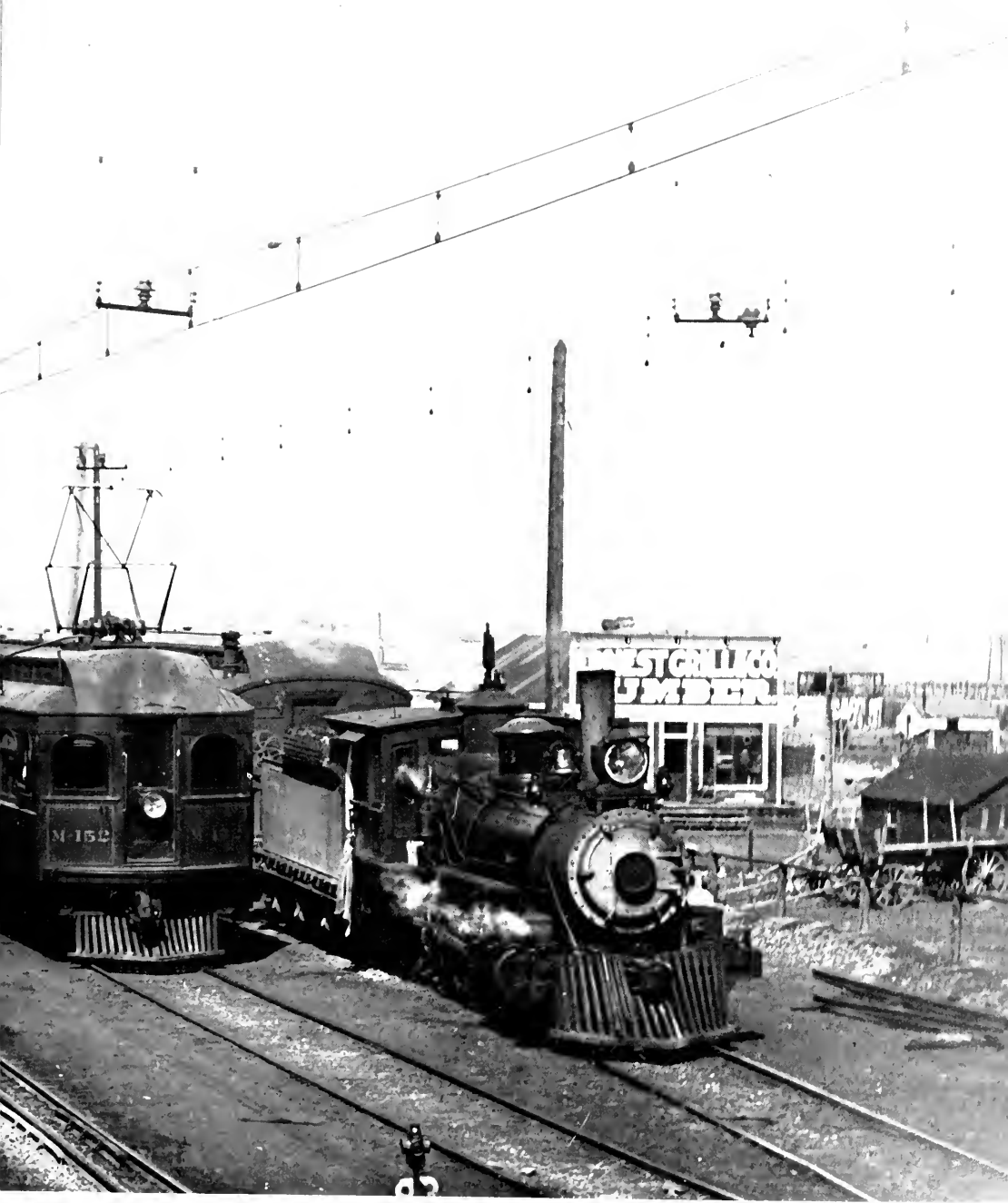
schedules with those of the parent C&S. The two interurban cars, en route to and from Denver, are meeting the C&S's Lafayette Stub local, powered by 4-4-0 No. 303. The dual-gauge track was employed for mixed-gauge freights transporting ore concentrates from the Denver, Boulder & Western interchange at Boulder to the smelter in Denver. BOULDER HISTORICAL SOCIETY.
