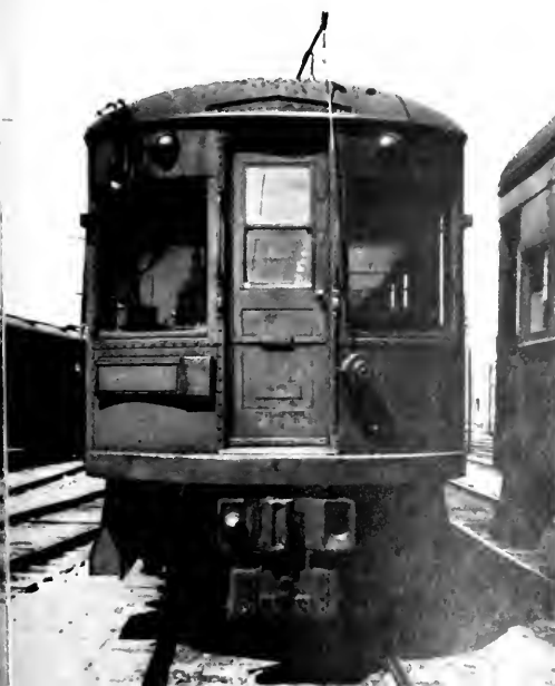
A close-up shows one type of fully automatic coupling, in interurban service on the Baltimore & Annapolis. WILLIAM D. MIDDLETON.
