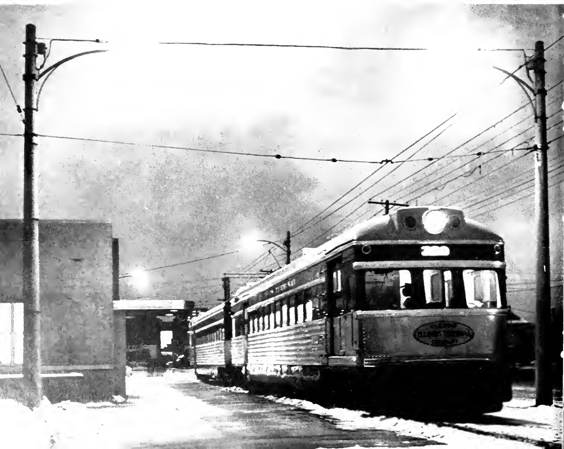
The interurban sleeping cars introduced by Illinois Traction in 1910 featured such advantages as upper-berth windows, extra-long berths, and individual safety deposit boxes. The Edwardsville was built by the St. Louis Car Company in 1913. WILLIAM J. CLOUSER COLLECTION.
