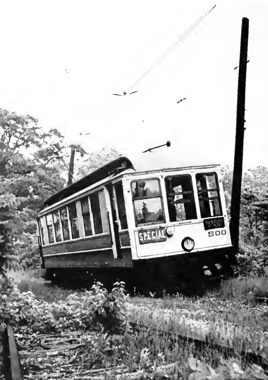
Connecticut Company officers and other distinguished personages rode about the system in high style aboard business car No. 500, built in 1904 by the J. G. Brill Company. The car's interior was finished in hand-carved oak, provided with a lavatory and steward's galley, and furnished with broadloom carpeting and wicker lounge chairs. After the end of Connecticut Company electric passenger service, No. 500 became the première car of the Branford Electric Railway museum, where these photographs were taken in 1959. BOTH PHOTOS: WILLIAM D. MIDDLETON.
