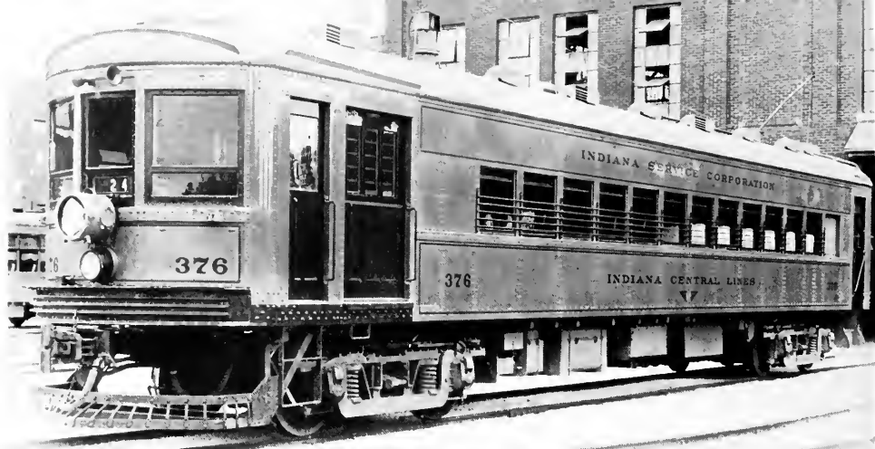
Interurban car architecture of the heavy steel car period tended to straightforward, functional design, and rarely were the results more pleasing than in the case of this Indiana Service Corporation combine, one of five constructed by the St. Louis Car Company in 1926. WILBOURNE B. COX COLLECTION.
