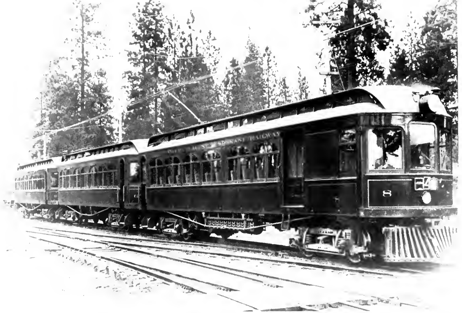
Brill-built combine 8 and trailers 61 and 62 rested at Coeur d'Alene in 1908. The trailers had observation platforms, and trolleys for standby lighting. LEROY O. KING JR. COLLECTION.
