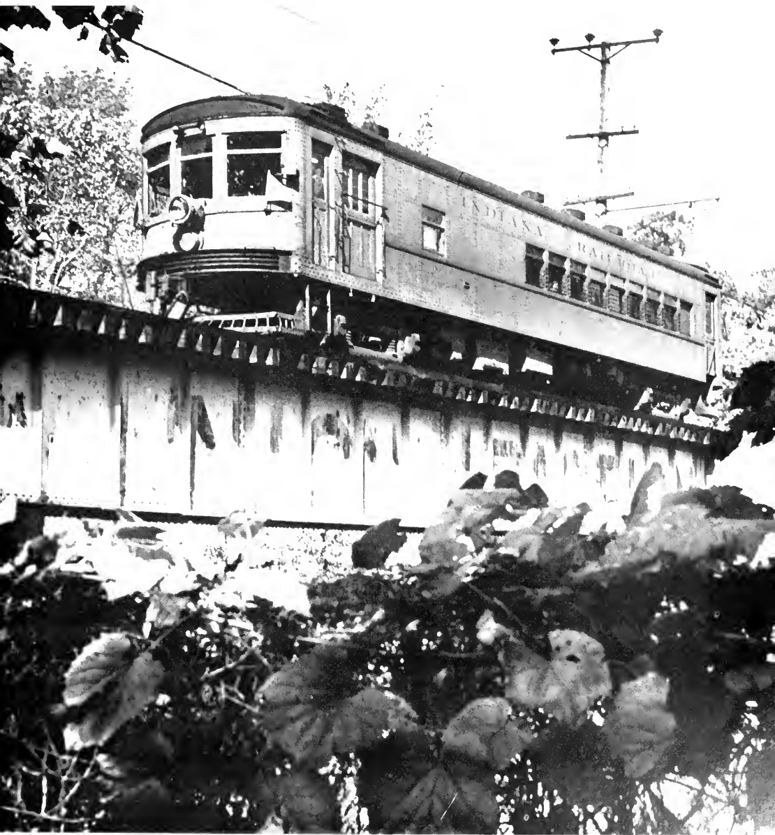
In 1935 IRR secured two Railway Post Office contracts, between Fort Wayne-New Castle and Indianapolis-Peru, given up by the Nickel Plate Railroad. To operate the service four former Indiana Service Corporation combines were rebuilt with RPO compartments. A fan excursion brought the 376 to the White River bridge near Anderson. The Union Traction name was still visible on the bridge.
