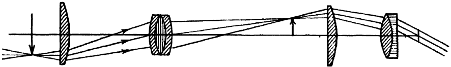
FIG. 27 TERRESTRIAL EYEPIECE WITH TRIPLE CEMENTED ERECTING LENS
