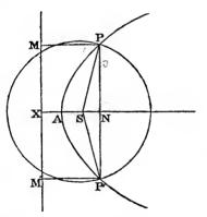
such that the ratio of SA to AX may be equal to the eccentricity. Then A is the vertex.
