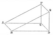
any two points P and Q in the former plane at right angles to AB, and let PC and QD be perpendiculars to the plane of projection. Then since AP and BQ are in a constant ratio to their projections AC and BQ, the rectilinear figure APQB is in the same constant ratio to its projection ACDB.
