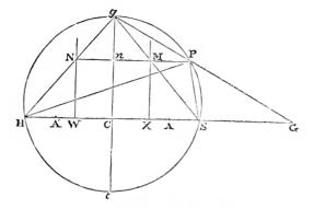
It is hence evident that any triangle may be projected by parallel lines into an equilateral triangle; and in like manner that any parallelogram may be projected into a square.
