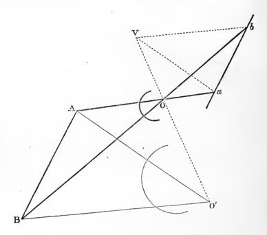
To project a given angle AOB in the primitive plane into an angle of given magnitude  $\alpha$ , let the arms of AOB meet the unprojected line in a and b; and upon ab describe in the vertex-plane a circular segment aVb containing an angle equal to  $\alpha$ . Then the vertex V may be taken at any point on this segment.
