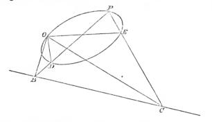
d. If a straight line PDB turning about a fixed point P meet the arms of a constant angle BOD, which turns about a fixed point O, in B and D; then if the point B moves along a straight line BC, the point D describes a conic through O and P. For when BC is the line at infinity the locus of D is evidently a circle through O and P; and therefore by reversion, the locus of D in the general case is a conic through O and P.
