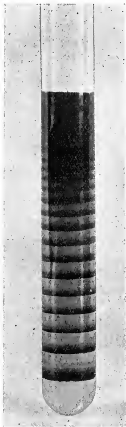
FIG. 11.—Adsorptive stratification of silver bichromate in an agar gel. (Bradford, Biochemical Journal. )
