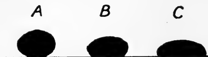
FIG. 5.—Form assumed by mercury globules under different electrical states. B is a mercury globule immersed in dilute \text{H}_2\text{SO}_4 . It assumes a more spherical form A when connected with the negative pole of a battery, while connection to the positive pole reduces surface tension as shown at C .
