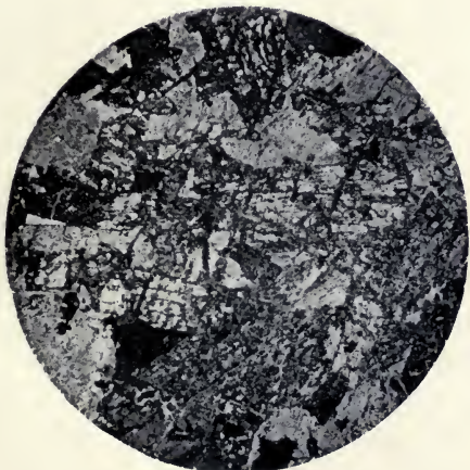
Photomicrograph of CHINA-CLAY ROCK from Treviscoe, St Stephens, between crossed nicols ( \times 12 diam.).
