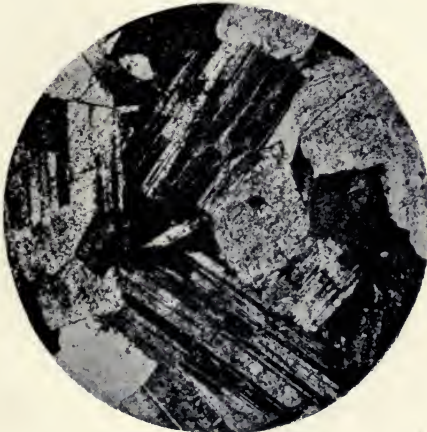
Photomicrograph of purple CHINA STONE from St Dennis, between crossed nicols ( \times 27 diam.).
