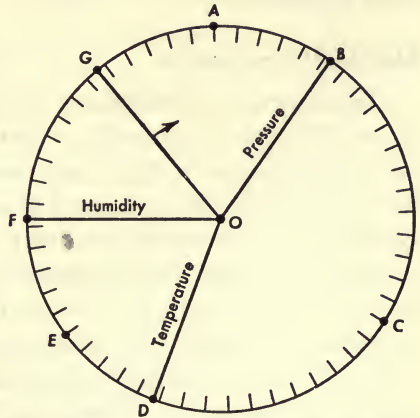
Fig. 68. A contactor arm sends radio signals steadily back to ground indicating pressure, temperature, and humidity at various elevations
