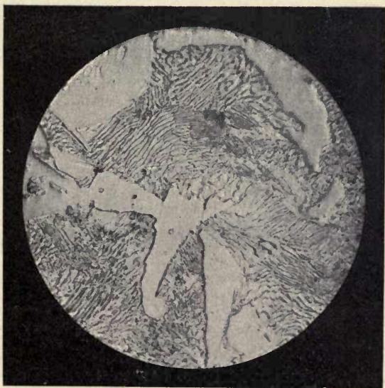
FIG. 140.—White pig-iron. Bright cementite in ground mass of pearlite.
