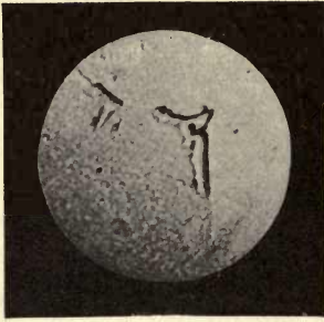
FIG. 129.—Forged iron containing 0.024 per cent. of carbon. Lamellæ of cementite surrounded by ferrite.
