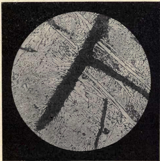
FIG. 143.—Grey pig-iron. Same material as in Fig. 142. Shows the lamellar structure of the pearlite.
