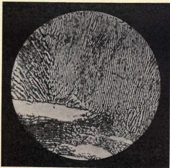
FIG. 156.—Lamellar pearlite and free cementite (bright).
