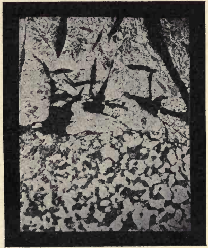
FIG. 151.—Same material as in Fig. 150 after annealing. The carbon has passed from the grey into the pure iron, so that the latter has become richer in pearlite.
