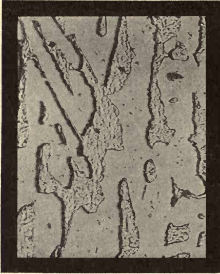
FIG. 157.—Structurally free cementite with ferrite.
