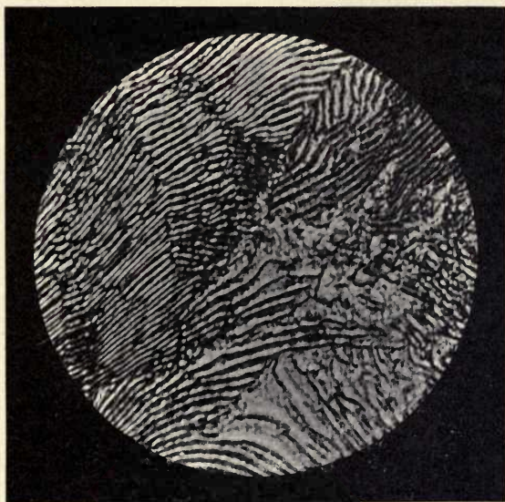
FIG. 131.—Eutectic steel. Lamellar pearlite.
