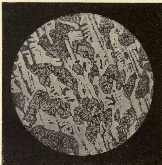
FIG. 152.—White pig-iron, quenched. Large white areas—cementite. Black patches—troostite. Ground mass— austenite-martensite.
