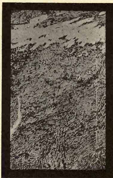
FIG. 132.—Hyper-eutectic steel. Free cementite surrounded by lamellar pearlite.
