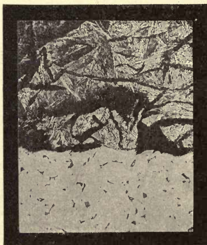
FIG. 150.—Upper part—grey pig-iron. Lower part—pure ingot-iron with a little pearlite.
