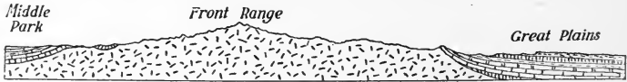
FIG. 125.—Section to show the arrangement given to the rocks by the uplifting of the Rocky Mountains. The base-line corresponds to sea-level. Altitudes: in Middle Park, 8,000 feet; crest of mountain, 13,500 feet; at the edge of the Plains, 5,500 feet.
