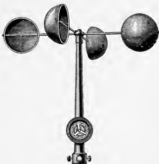
FIG. 177.—The anemometer. Inside the upright is a spindle to which the cross-bars are fastened. The wind pushes harder against the hollows of the cups than against the outsides, and thus turns the spindle. The stronger the wind, the faster the spindle whirls. A counting machine below is worked by the spindle and makes a record.
