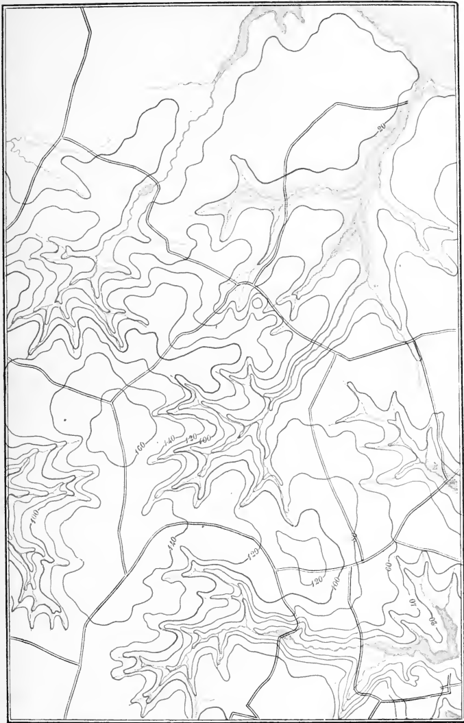
FIG. 44.—Part of Virginia, bordering the Potomac River. Scale, 1 inch = 1 mile. Contour interval, 20 feet. Streams are developing their valleys by eating backward into the land, but tracts of the original plain remain. Roads find easy grades on the divides. See Sec. 50.
