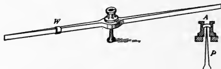
FIG. 186.—A magnetic needle, with a cross-section to show the mode of hanging. P , pivot; A , cap of agate with hollow beneath to rest on the pivot; W , adjustable weight to counteract the dipping tendency (page 277).
