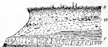
FIG. 2.—Ideal cutting, or "section," showing soil ( s ), the mantle of waste ( w ), and bed-rock ( r ).
