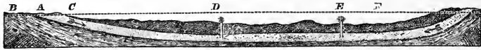
FIG. 75.—Ideal section of a valley, showing the principle of artesian wells. A , a porous rock; B , C , impervious rocks; F , height of the water-level in A ; D , E , artesian wells, made where the ground is lower than F .
