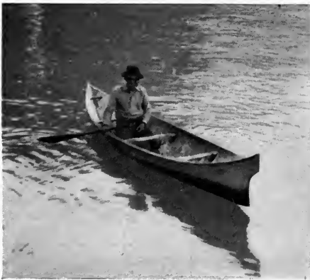
FIG. 252.—A dug-out, a boat carved from a log and propelled by a paddle; Alaska.
