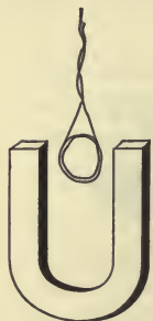
FIG. 107.— As long as the coil rotates between the poles of the magnet, current flows.
