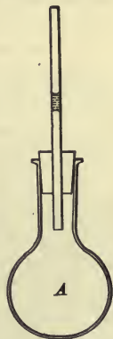
FIG. 3. — As the air in A is heated, it expands and forces the drop of ink up the tube.
