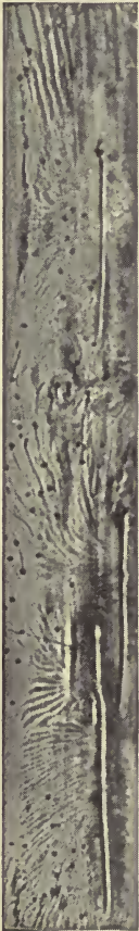
FIG. 344. — A piece of wood destroyed by borers.
