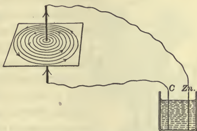
FIG. 100.— A wire through which current flows is surrounded by a field of magnetic force.
