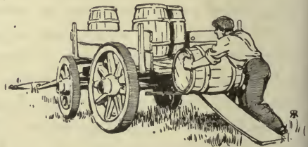
FIG. 153.—Rolling barrels up a plank.
