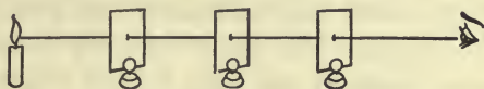
FIG. 112.—The candle cannot be seen unless the three pinholes are in a straight line.
