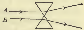
FIG. 127. — Rays of light are diverged and do not come to any real focus.
