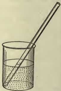
FIG. 246. — The water in the tube is at the same level as that in the glass.
