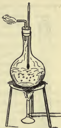
FIG. 8. — Determining one of the fixed points of a thermometer.
