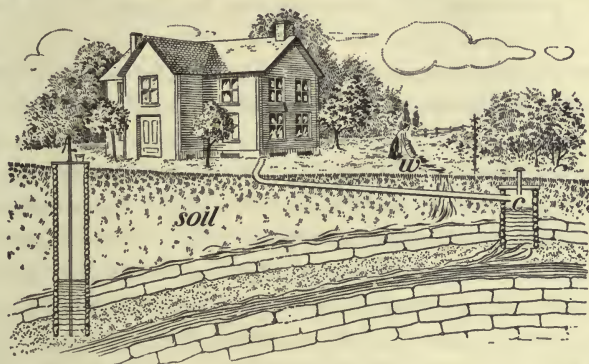
FIG. 72. — Showing how drinking water can be contaminated from cesspool (c) and wash water (w).
