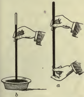
FIG. 248.— The air supports a column of mercury 30 inches high.
