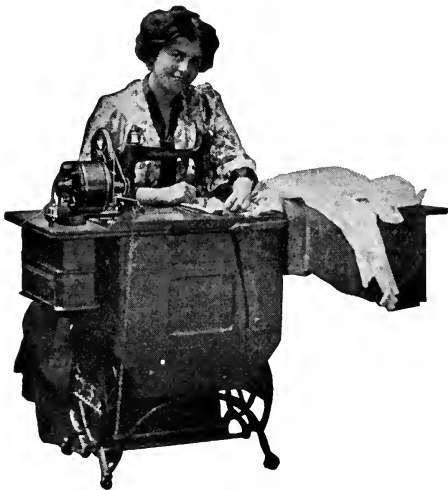
FIG. 105. — A motor runs the sewing machine.
