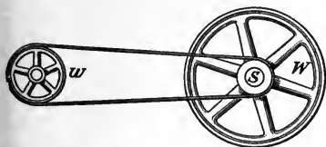
FIG. 176. — By means of a belt, motion can be transferred from place to place.
