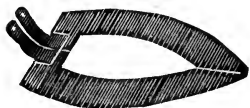
FIG. 77. — The fine wires are strongly heated by the current which flows through them.
