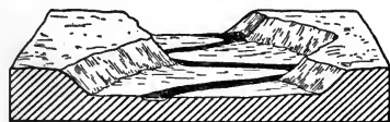
FIG. 237.—As a river approaches base level, it widens its valley by side cutting.
