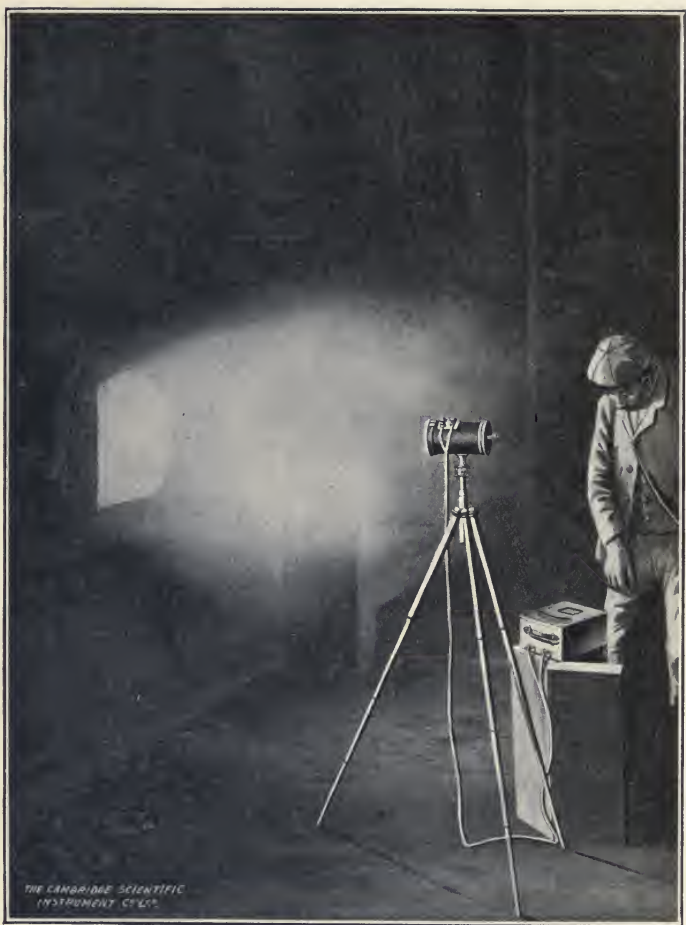
Taking Temperature of a Gas Retort with a Fery Radiation Pyrometer. Frontispiece. ]
