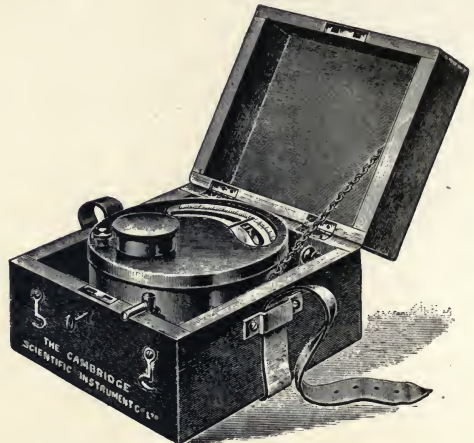
FIG. 24.—Millivoltmeter, Portable Form.
