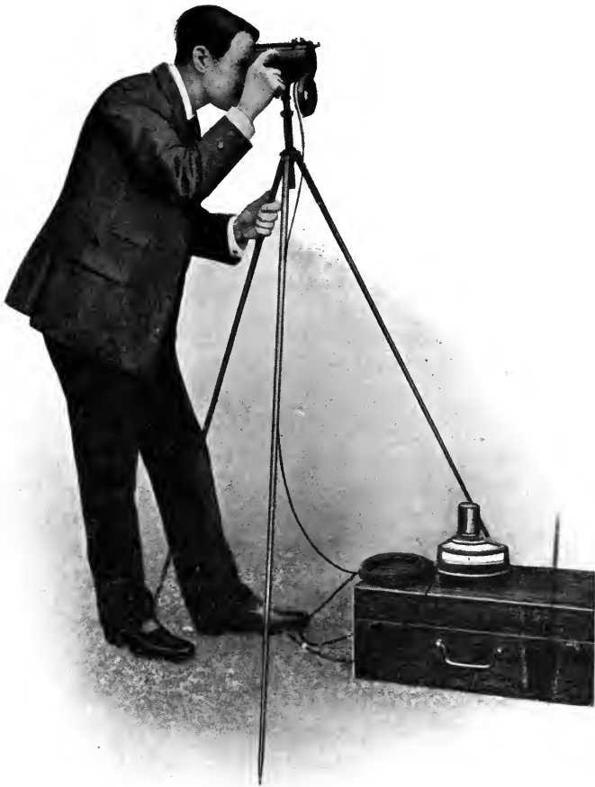
FIG. 35.—Sighting a Fény Radiation Pyrometer.
