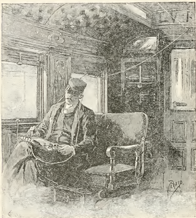
Interior of a Car on the Lehigh Valley Railroad, showing the Method of Operating the Train Telegraph.
