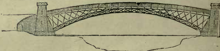
CAST IRON BRIDGE AT CRAIGELLACHIE.
