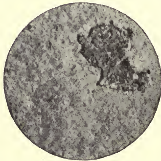
FIG. 16 (magnified).—Rust produced by dilute hydrochloric acid on an almost undamaged surface of iron plate. The large patch shows where the rust has flaked off.
