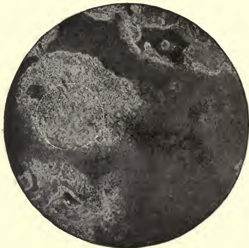
FIG. 1 (natural size).—Rust on rolled sheet iron, scoured with pumice; produced by falling drops of water constantly evaporated.
