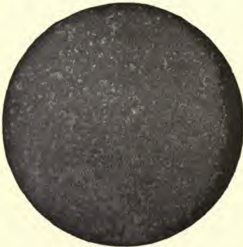
FIG. 34 (natural size).—Rolled sheet iron scoured with pumice and exposed for five minutes to the action of concentrated hydrochloric acid. The holes have been eaten away by rust.
