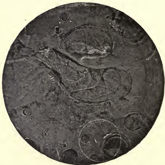
FIG. 43 (natural size).—Effect of water on wet paint, with immediate formation of rust.
