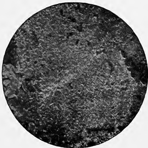
FIG. 9 (natural size).—Rust produced on rolled iron plate by the action of concentrated hydrochloric acid for twenty-four hours.
