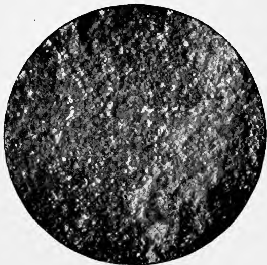
FIG. 27 (magnified).—Thoroughly corroded iron plate: atmospheric action.
