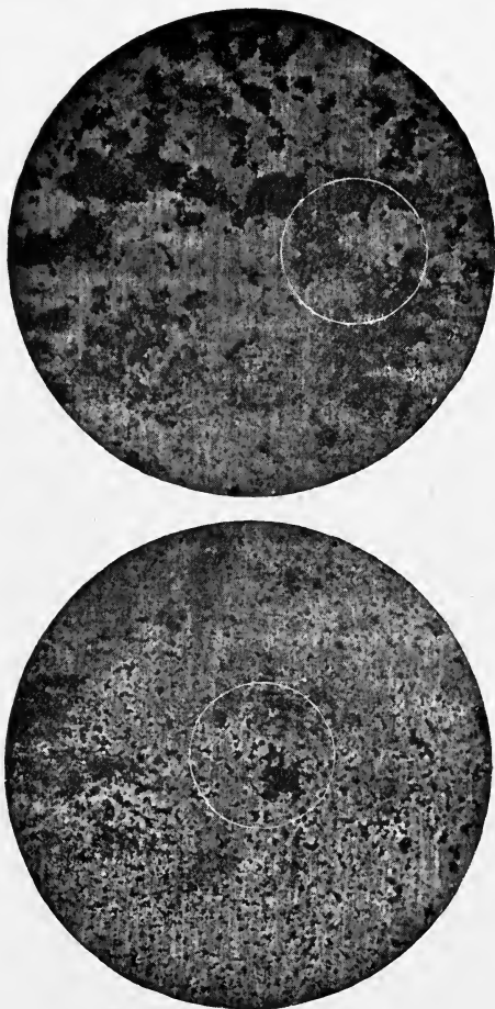
FIGS. 30 and 31.—Rust pittings in tinned sheet iron stored for ten years in a cellar. The black patches are the rust, the lighter portions indicating the clean metal.
