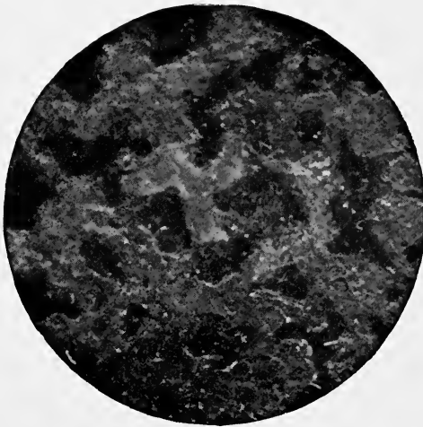
FIG. 40 (magnified).—Blisters, formed by warmth, in a red lead paint poor in varnish, covering a bottom coat rich in oil.
