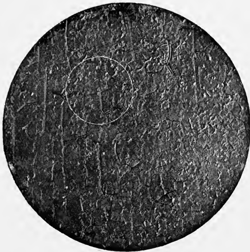
FIG. 41 (natural size).—Cracks in an oil paint, with another, intermediate layer.
