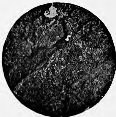
FIG. 25 (natural size).—Sheet of iron perforated by rust; the white patches are the holes, and the dark lines show the flakes of rust in the act of peeling off.
