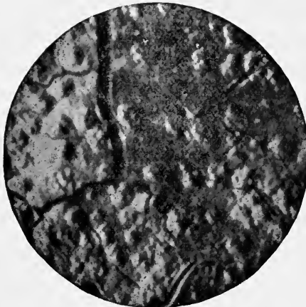
FIG. 50 (magnified).—Blisters and cracks caused by heating a layer of oil paint.
