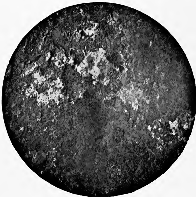
FIG. 23 (natural size).—Rust produced on iron plate through ordinary wear and condensed moisture.
