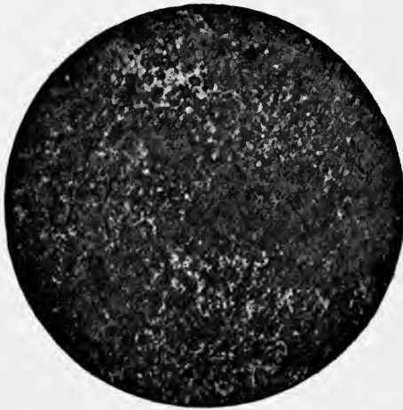
FIG. 8 (natural size).—Rust produced on rolled iron plate by the action of concentrated hydrochloric acid for twenty-four hours.
