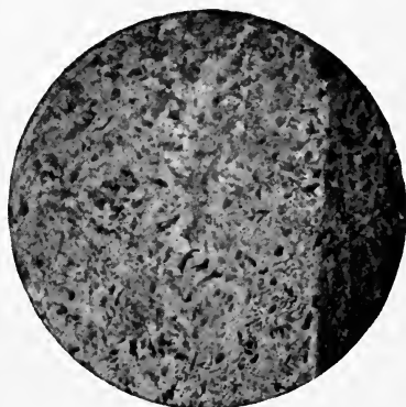
FIG. 10 (natural size).—Rust on rolled iron plate with defective surface, produced in five minutes by the action of dilute hydrochloric acid.
