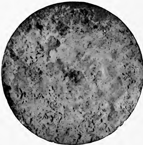
FIG. 2 (magnified).—Rust on rolled sheet iron, scoured with pumice; produced by falling drops of water constantly evaporated.
