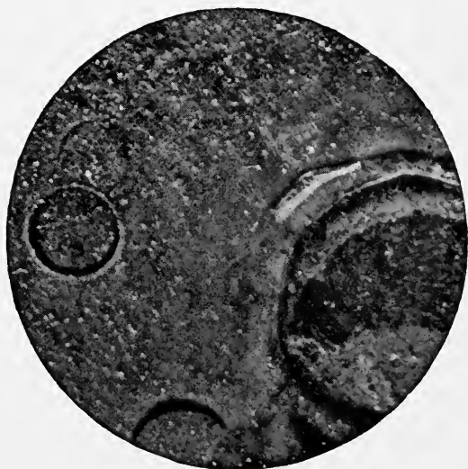
FIG. 44 (magnified).—Effect of water on wet paint, with immediate formation of rust.
