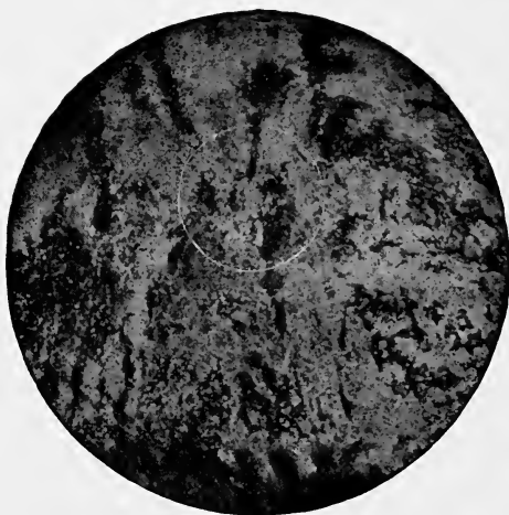
FIG. 6 (natural size).—Rust on rolled iron plate, produced by a single application of water left to dry on.
