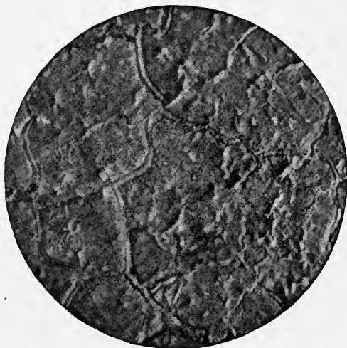
FIG. 42 (magnified).—Cracks in an oil paint, with another, intermediate layer.
