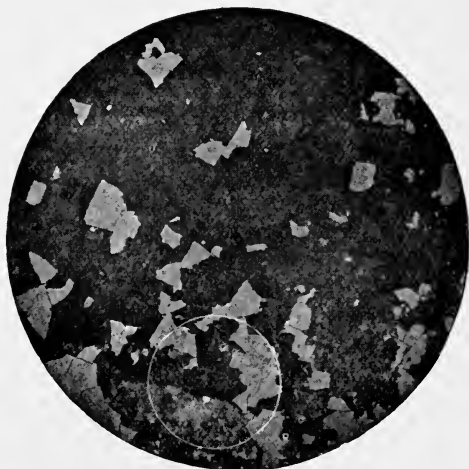
FIG. 61 (natural size).—Peeling anti-fouling composition after six months' immersion in water.
