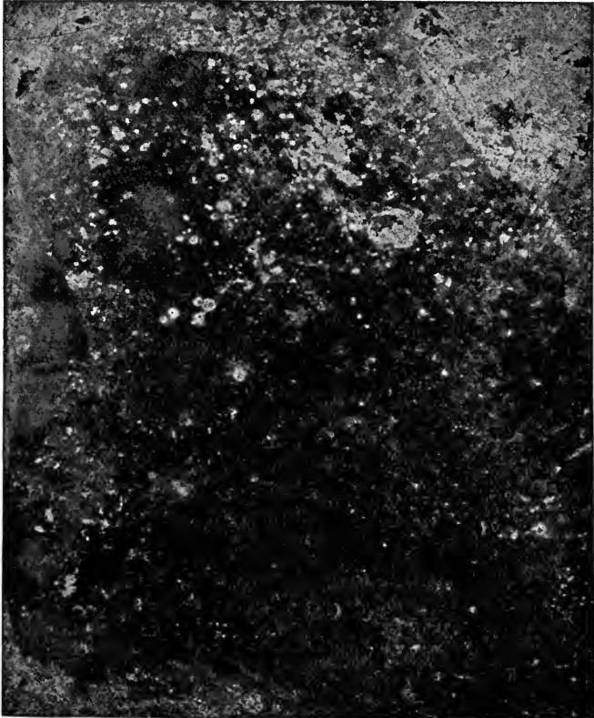
FIG. 3 (natural size).—Rust produced on rolled iron plate in twelve hours by moistening with water and leaving it to dry.
