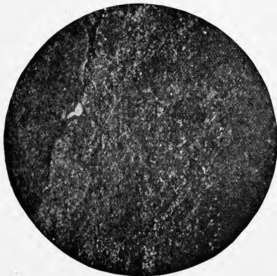
FIG. 24 (natural size).—Rust developed on sheet iron in ordinary use as a stove pipe.
