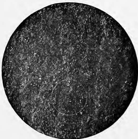
FIG. 26 (natural size).—Thoroughly corroded iron plate : atmospheric action.
