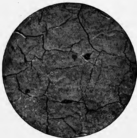
FIG. 60 (magnified).—Non-peeling anti-fouling composition after three months' immersion in water.
