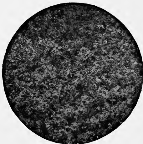
FIG. 35 (magnified).—Rolled sheet iron scoured with pumice and exposed for five minutes to the action of concentrated hydrochloric acid. The holes have been eaten away by rust.
