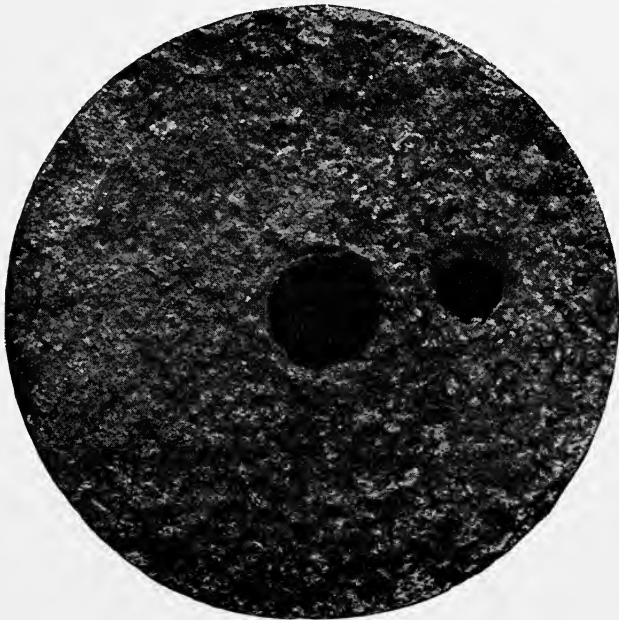
FIG. 28 (natural size).—Thick incrustation of rust developed on a wrought-iron disc by exposure in the open air.
