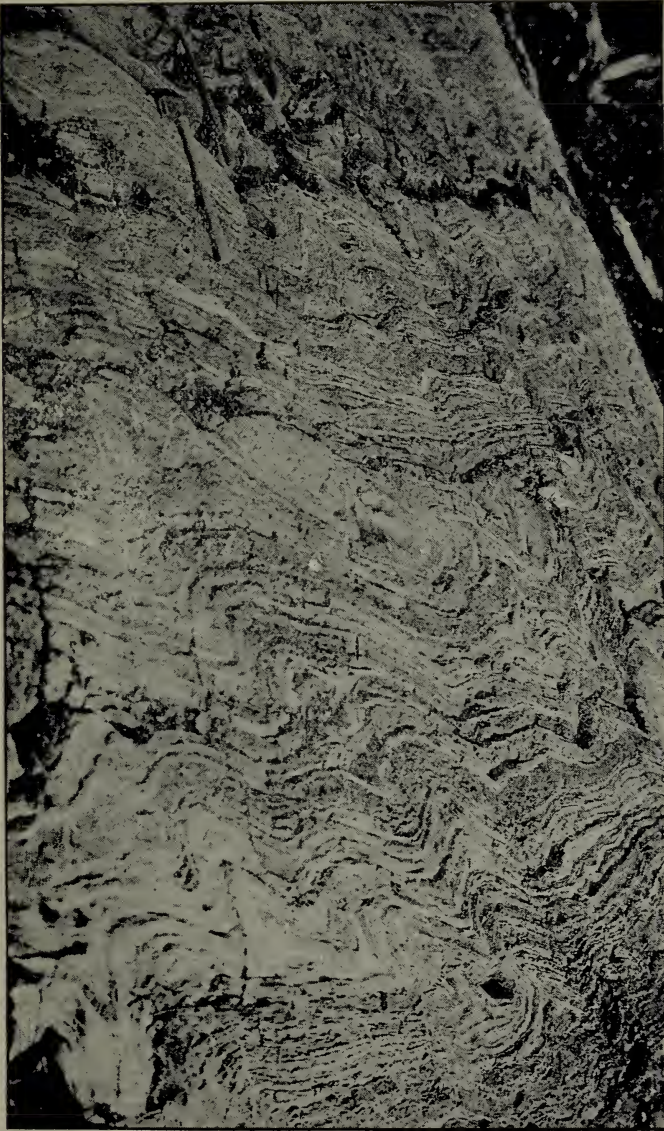
CONTORTED JASPILYTE, ON THE N. SLOPE OF THE NORTH RIDGE, NEAR THE TOWER MINE. (THE HAMMERS LIE ON THE LAMINÆ OF SILICEOUS GREEN SCHIST.) (P. 54)
