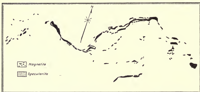
FIG. 19.—Scandinavian ore deposits showing linear arrangement of magnetic ore-bodies. (Stützer.)
