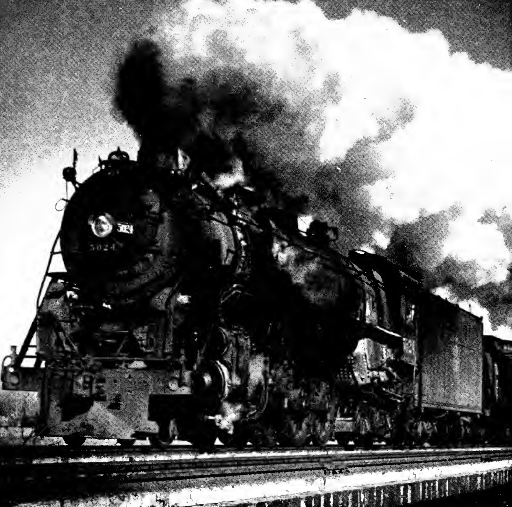
14 Rock Island's 5000-class 4-8-4's, great among the high-speed tonnage haulers in World War II, now replaced by diesels.
