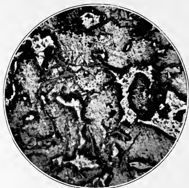
FIG. 71.—Cast Iron with Phosphide Eutectic.
