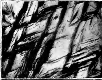
FIG. 68.—Austenite and Martensite.
