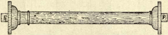
Fig. 10.—Wood Pattern for Moulding Cast-iron Column.
