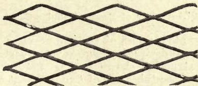
Fig. 191.—Enlarged View of Expanded Metal Lathing.
