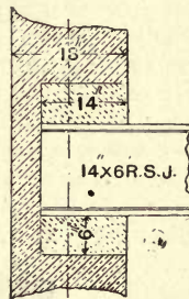
Fig. 102.—Fixing of Girder in Wall, Section.
