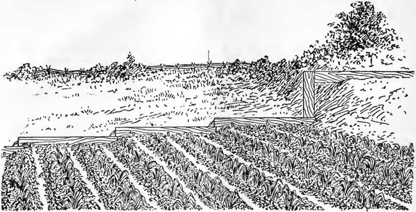
FIG. 17.—Furrow irrigation on a slope with stepped flumes and drop.
