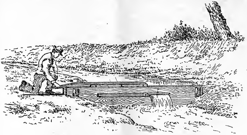
FIG. 2.—Measurement of a brook by the miner's inch method.
