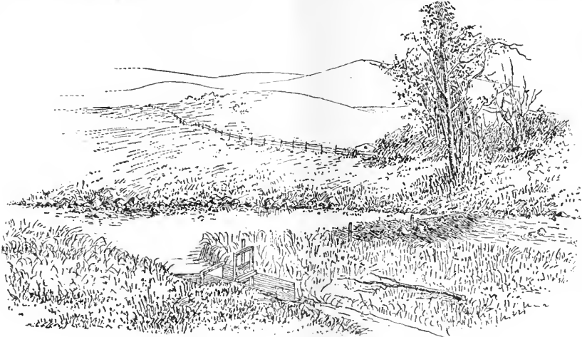
FIG. 3.—Diverting a small stream, showing brush dam and headgate.
